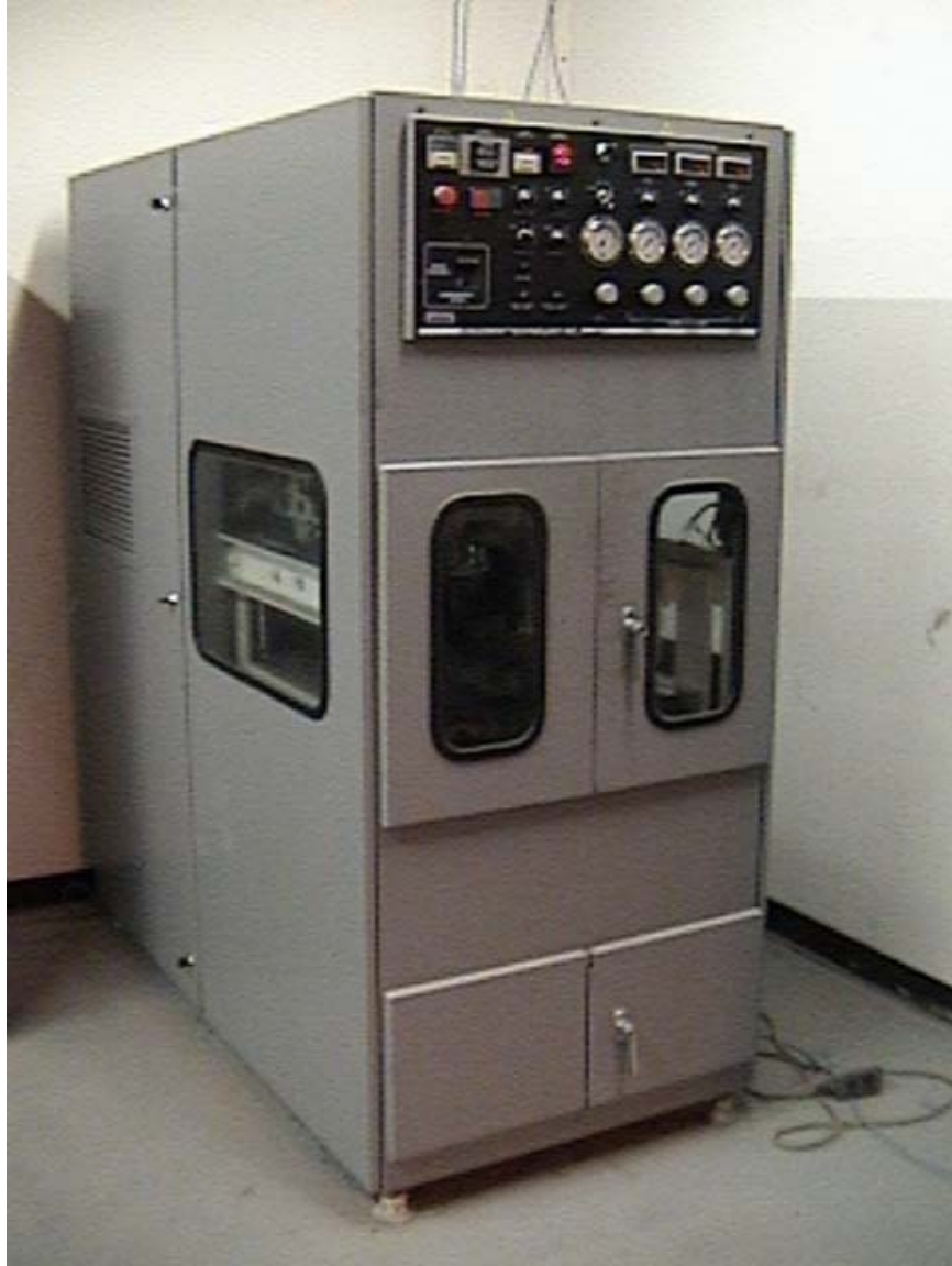
Figure 1 – Asphalt Pavement Analyzer
