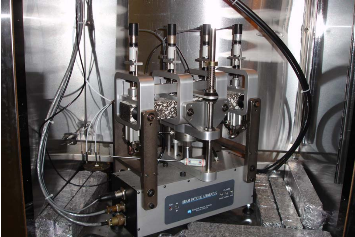
Figure 3 – Flexural Beam Fatigue Device
