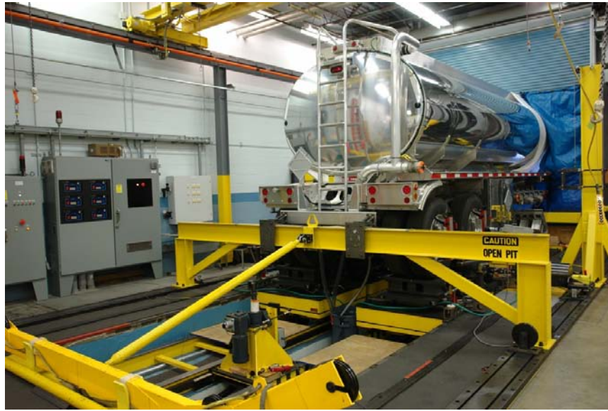
Figure 2-2. Photo. LBT tanker in kinematics and compliance (K&C) testing
