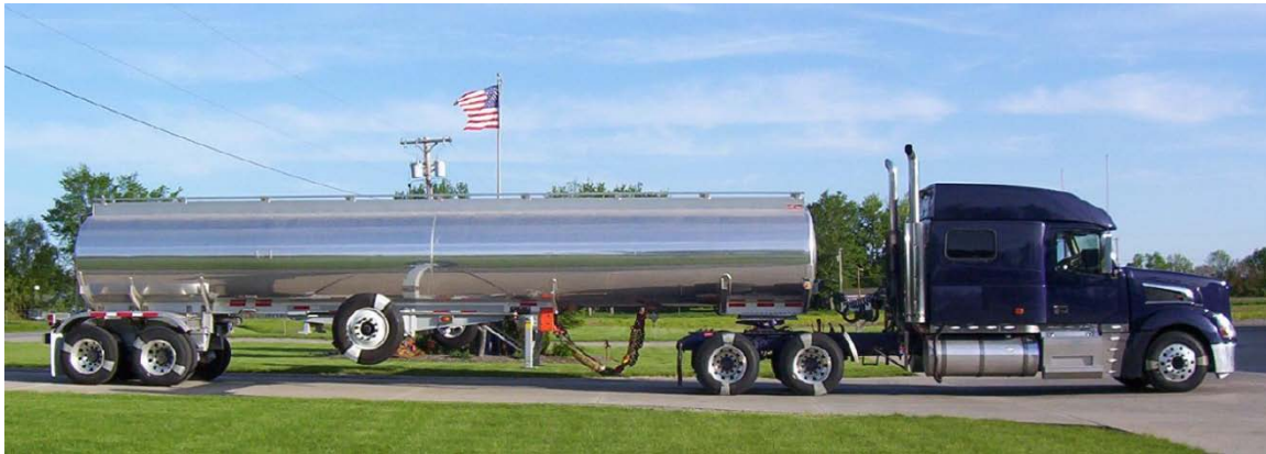
Figure ES-1. Photo. This tractor and tank semitrailer were used in the experiments. In this phase's work, two different suspensions were mounted under the semitrailer. Experiments with different tires and semitrailer CG heights were conducted in a previous phase.
