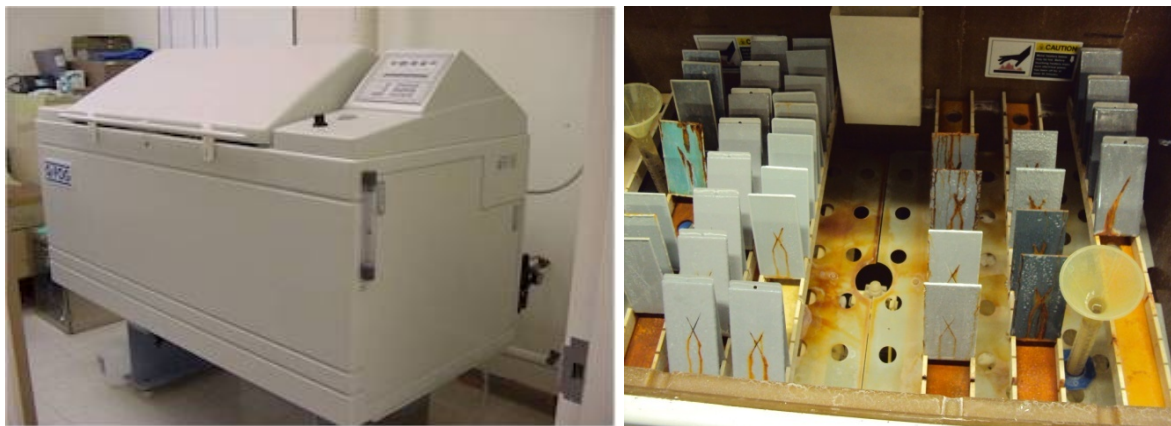
Figure 4.3 Salt Fog Test Setup.
