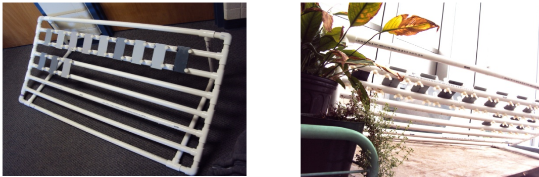
Figure 4.10 Atmospheric Exposure Testing Setup.
