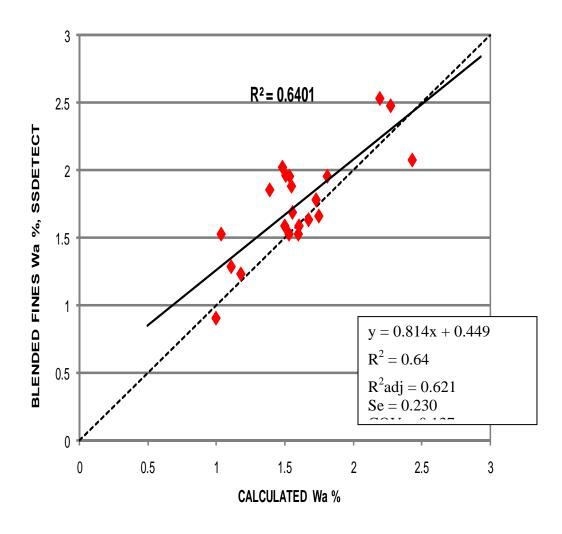
Figure 8 Blended-Calculated against SSDetect Wa%
