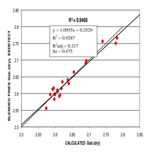
Figure 5 Blended-Calculated against SSDetect Gsb (dry)
