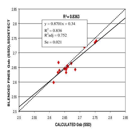
Figure 6 Blended-Calculated against SSDetect Gsb (SSD)
