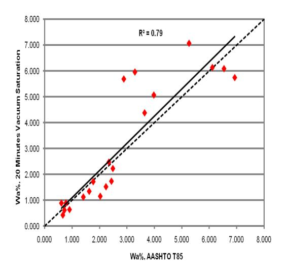
Figure 19 AASHTO T-85 against 20 Minutes Vacuum Saturation Test for Wa%
