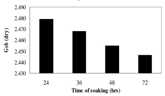
Figure 25 Gsb (dry) test results over 24, 36, 48 and 72 hours of soaking periods
