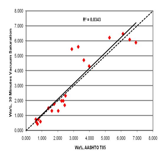
Figure 20 AASHTO T-85 against 30 Minutes Vacuum Saturation Test for Wa%
