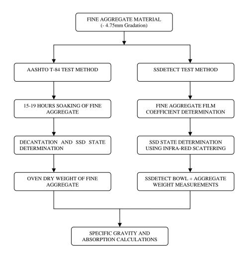
Figure 1. Flow chart indicating the processes carried out for the AASHTO T 84 against the SSDetect
