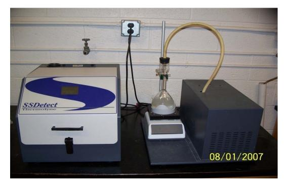
Figure 5. The SSDetect with AVU unit
