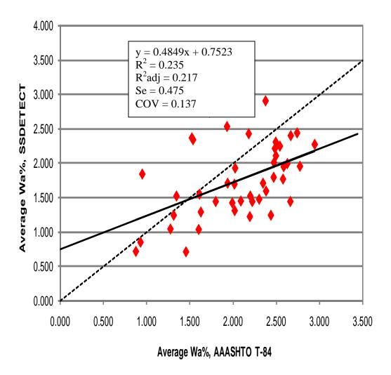
Figure 4 AASHTO T-84 against SSDetect Water Absorption (Wa %)
