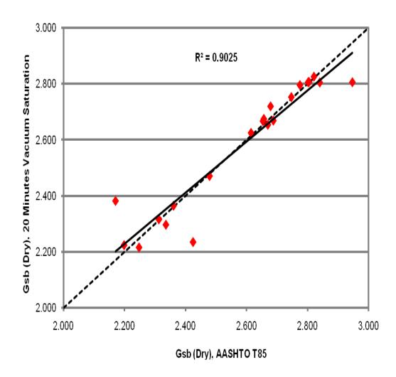
Figure 10 AASHTO T-85 against 20 Minutes Vacuum Saturation Test for Gsb (dry)
