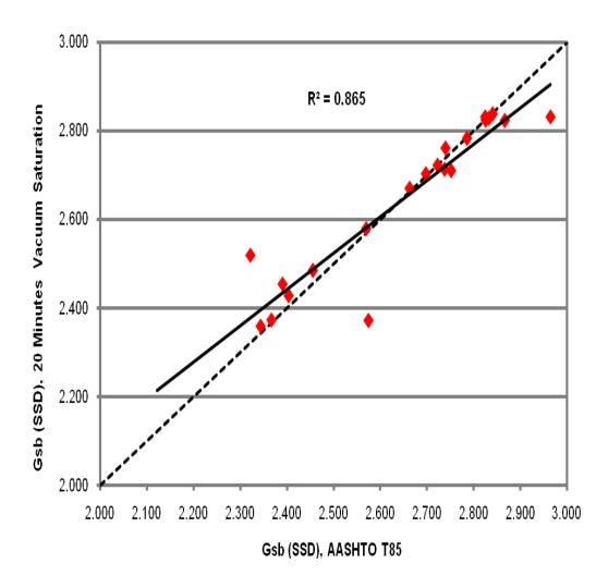
Figure 13 AASHTO T-85 against 20 Minutes Vacuum Saturation Test for Gsb (SSD)
