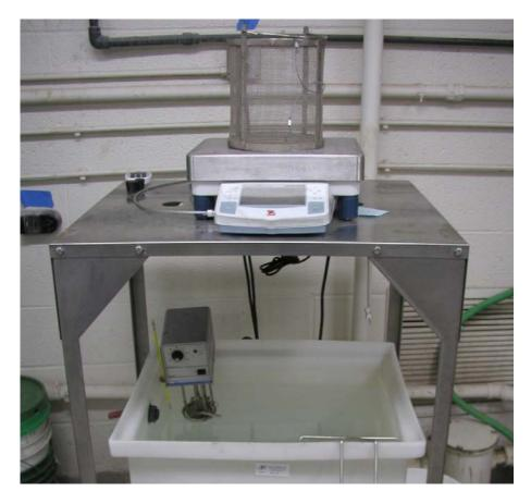
Figure 8. The set-up of the AASHTO T85
