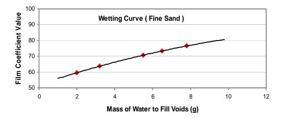
Figure 7 Film Coefficient Curve for the fine sand aggregate
