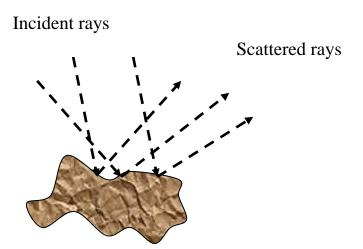
Figure 4. Scattering of light rays on an uneven surface (fine aggregate
