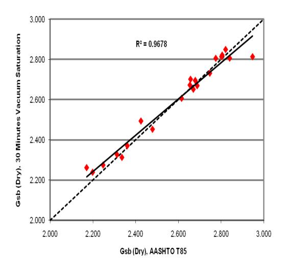
Figure 11 AASHTO T-85 against 30 Minutes Vacuum Saturation Test for Gsb (dry)
