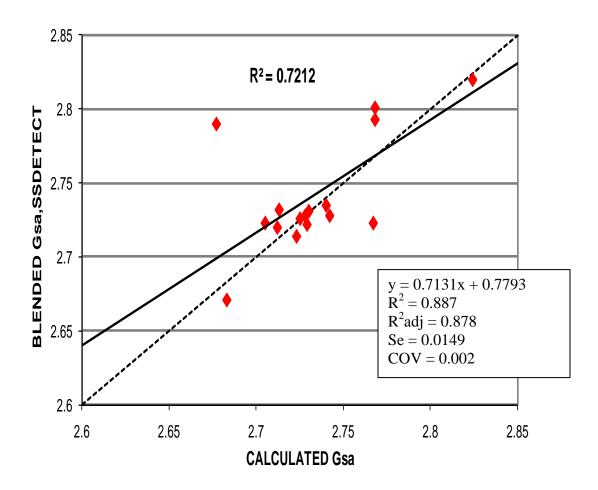
Figure 7 Blended-Calculated against SSDetect Gsa
