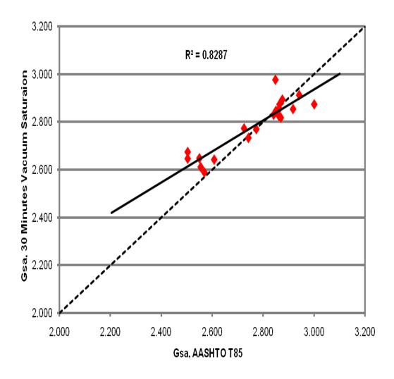
Figure 17 AASHTO T-85 against 30 Minutes Vacuum Saturation Test for Gsa
