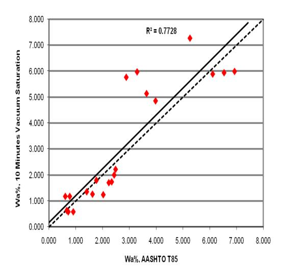
Figure 18 AASHTO T-85 against 10 Minutes Vacuum Saturation Test for Wa%
