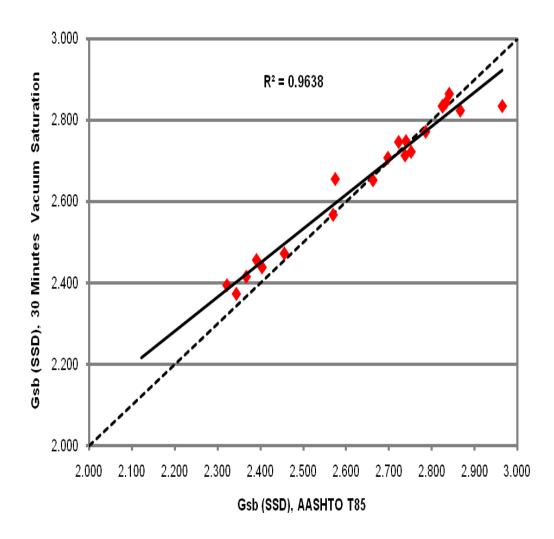
Figure 14 AASHTO T-85 against 30 Minutes Vacuum Saturation Test for Gsb (SSD)
