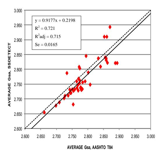
Figure 3 AASHTO T-84 against SSDetect Bulk Specific Gravity (Gsa)
