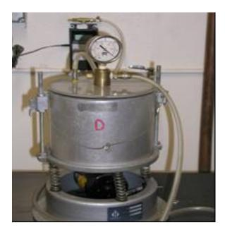
Figure 9. The Vacuum saturation apparatus used to expel the air in the coarse aggregate mass and force water into the pores of the aggregates
