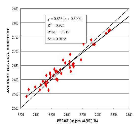
Figure 1 AASHTO T-84 against SSDetect Bulk Specific Gravity (dry)
