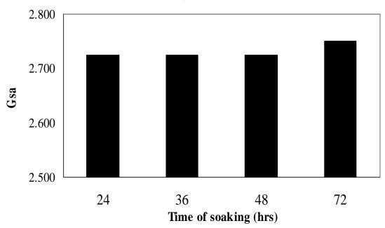
Figure 27 Gsa test results over 24, 36, 48 and 72 hours of soaking periods
