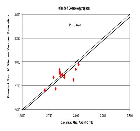
Figure 23 Gsa: Calculated Value against Single Test Value of 10 Minutes Vacuum Saturation Test
