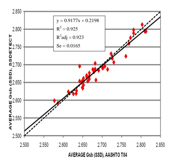
Figure 2 AASHTO T-84 against SSDetect Bulk Specific Gravity (SSD)
