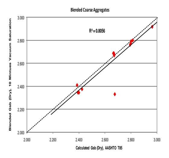
Figure 21 Gsb (Dry): Calculated Value against Single Test Value of 10 Minutes Vacuum Saturation Test
