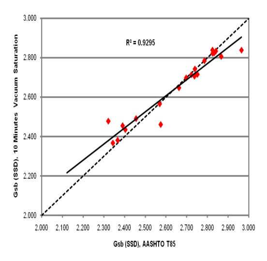
Figure 12 AASHTO T-85 against 10 Minutes Vacuum Saturation Test for Gsb (SSD)
