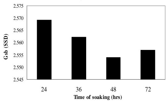
Figure 26 Gsb (SSD) test results over 24, 36, 48 and 72 hours of soaking periods
