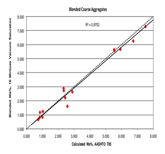
Figure 24 Wa%: Calculated Value against Single Test Value of 10 Minutes Vacuum Saturation Test
