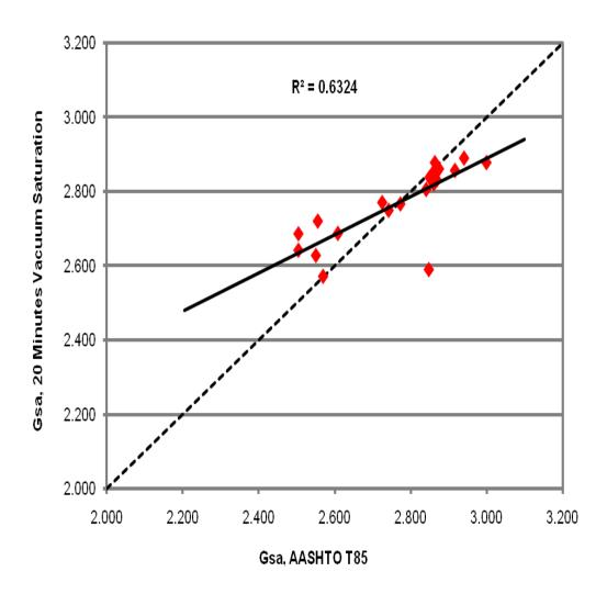
Figure 16 AASHTO T-85 against 20 Minutes Vacuum Saturation Test for Gsa
