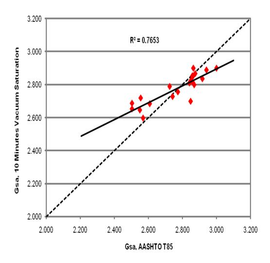
Figure 15 AASHTO T-85 against 10 Minutes Vacuum Saturation Test for Gsa
