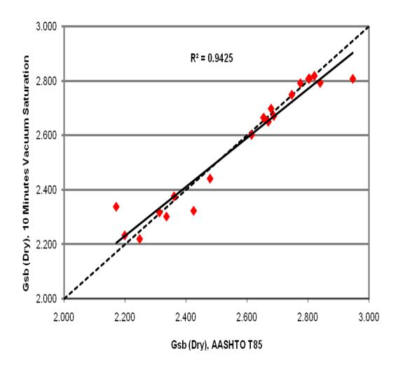
Figure 9 AASHTO T-85 versus 10 Minutes Vacuum Saturation Test for Gsb (Dry)
