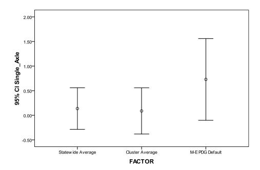
Figure 4.18 Error Bar Chart for Differences in Rigid Performance Life Based on Single Axle Load Traffic Inputs
