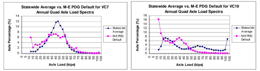
Figure G23. State Avg. vs. M-E PDG Default for Quad VC7 LS
