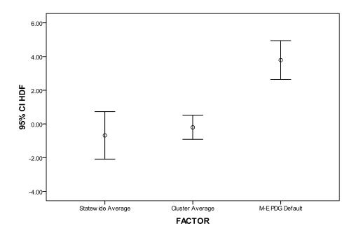
Figure 4.16 Error Bar Chart for Differences in Rigid Performance Life Based on HDF Traffic Inputs
