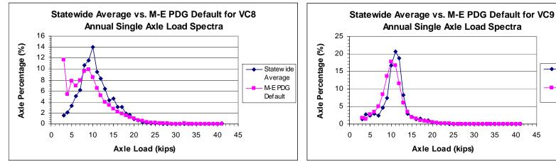
Figure G5. State Avg. vs. M-E PDG Default for Single VC8 LS
