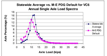
Figure G3. State Avg. vs. M-E PDG Default for Single VC6 LS
