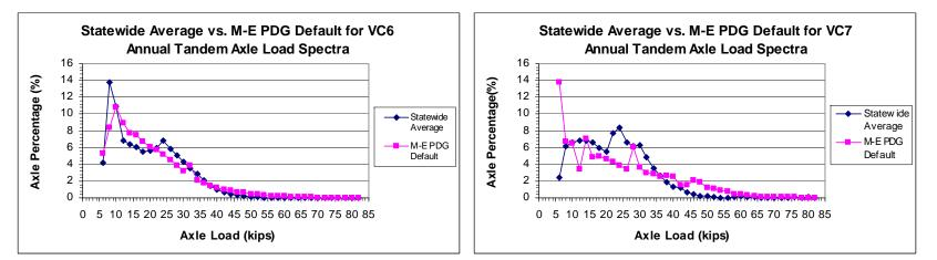
Figure G13.State Avg. vs. M-E PDG Default for TandemVC6 LS Figure G14.State Avg. vs. M-E PDG Default for TandemVC7 LS
