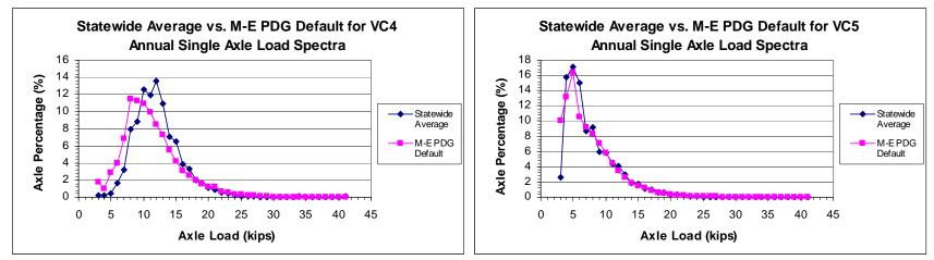
Figure G1. State Avg. vs. M-E PDG Default for Single VC4 LS
