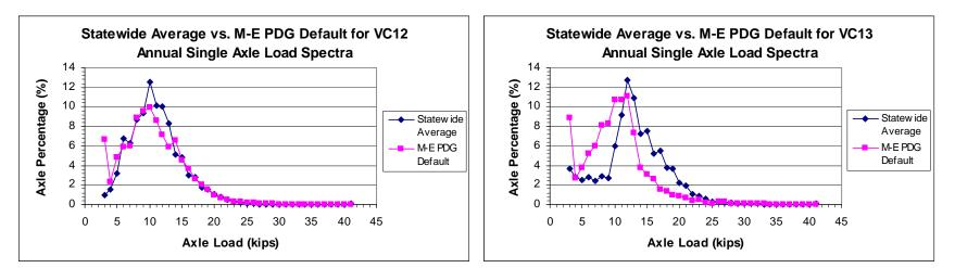
Figure G9. State Avg. vs. M-E PDG Default for Single VC12 LS Figure G10. State Avg. vs. M-E PDG Default for Single VC13 LS
