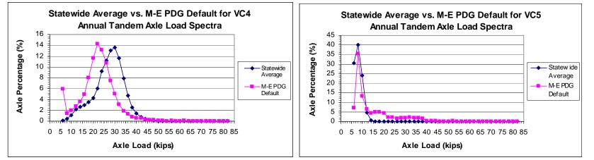
Figure G11.State Avg. vs. M-E PDG Default for TandemVC4 LS Figure G12.State Avg. vs. M-E PDG Default for Tandem VC5 LS
