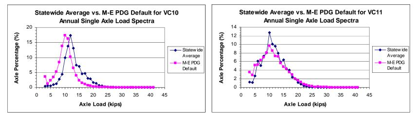
Figure G7. State Avg. vs. M-E PDG Default for Single VC10 LS Figure G8. State Avg. vs. M-E PDG Default for Single VC11 LS
