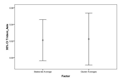
Figure 4.32 Error Bar Chart for Differences in Flexible Performance Life Based on Rutting Due to Tridem Axle Load Spectra Characterization
