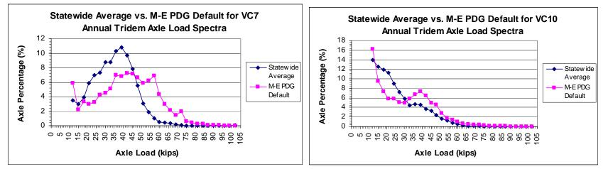
Figure G20.State Avg. vs. M-E PDG Default for Tridem VC7 LS Figure G21.State Avg. vs. M-E PDG Default for TridemVC10 LS
