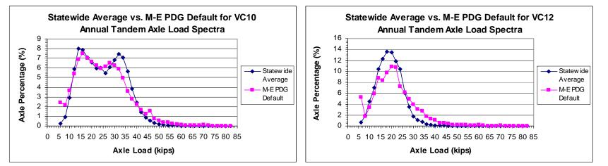
Figure G17.State Avg. vs. M-E PDG Default for TandemVC10 LS Figure G18.State Avg. vs. M-E PDG Default for TandemVC12 LS
