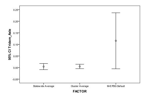
Figure 4.20 Error Bar Chart For Differences in Rigid Performance Life Based on Tridem Axle Load Traffic Inputs
