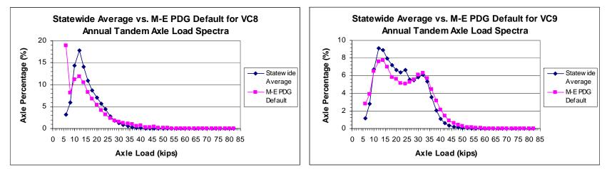
Figure G15.State Avg. vs. M-E PDG Default for Tandem VC8 LS Figure G16.State Avg. vs. M-E PDG Default for TandemVC9 LS
