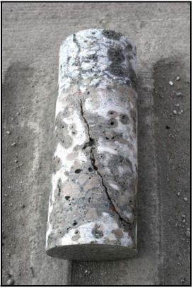
FIGURE 6 Contrast in Crack Width per Depth of Euro-Pavement Longitudinal Crack
