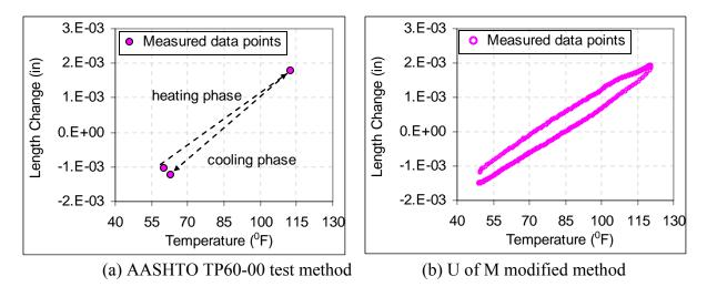
Figure 1 CTE Test Methods (AASHTO versus U of M)
