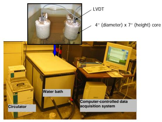
Figure 3 CTE Test Setup at U of M
