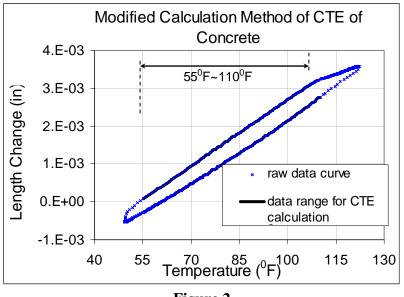
Figure 2 Calculation Method of CTE in the Modified Test Method
