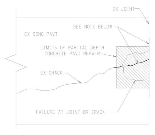
PARTIAL DEPTH CONCRETE PAVEMENT REPAIR DETAIL
