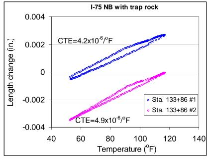
Figure 4 CTE of Cores with Trap Rock
