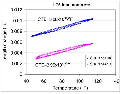
Figure 5 CTE of Lean Concrete Cores
