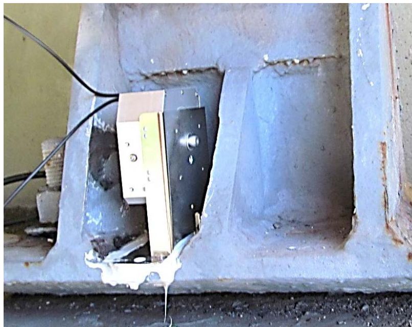
Figure 23. Tilt Meter at a Roller Support
