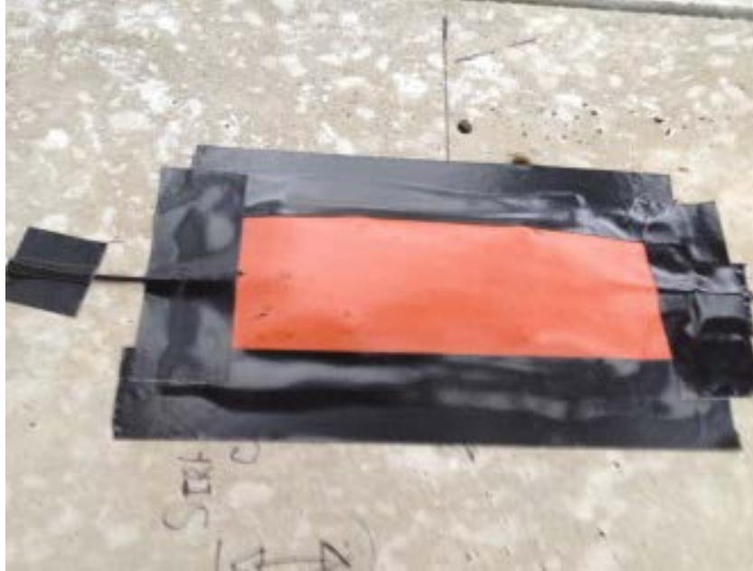
Figure 20. Strain Sensor with Protective Cover
