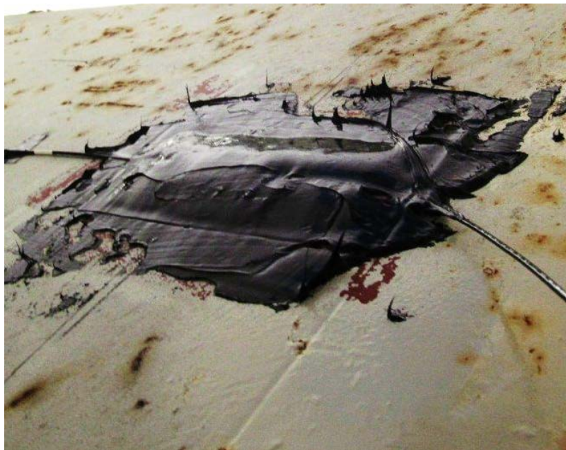
Figure 17. Strain Sensor Cover with the Protection Coating
