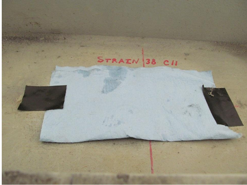
Figure 14. Rust Prevention: Used a Temporary Protective Covering
