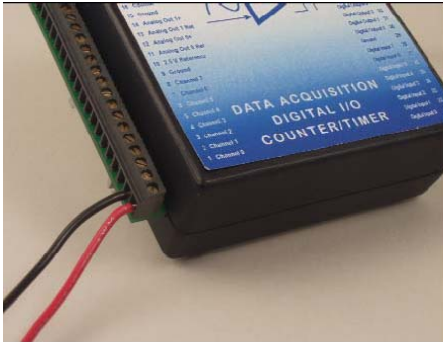
Figure 4 Connect Distance Input to Channel 0, Start Sensor to Channel 1
