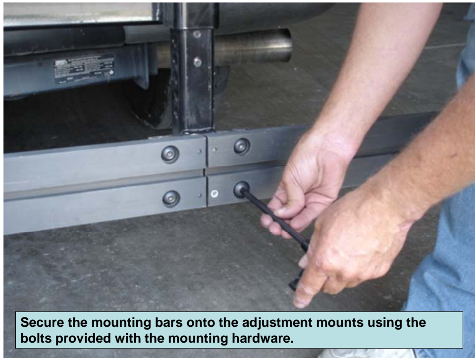
Figure 24 Secure Mounting Bars
