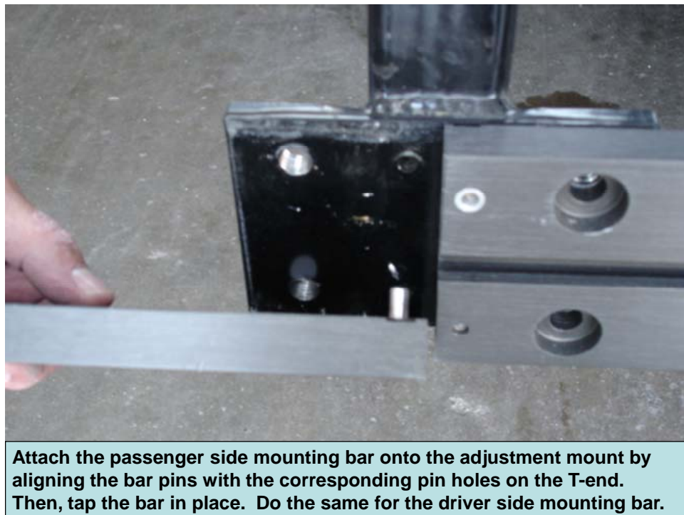
Figure 23 Attach Side Mount
