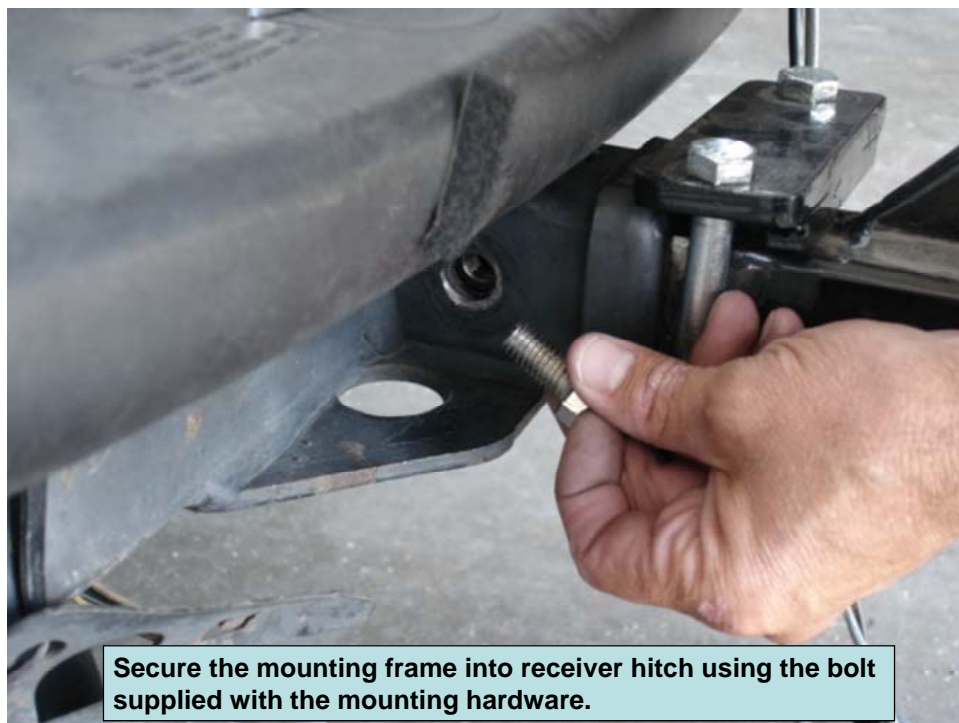
Figure 19 Secure Mounting Frame
