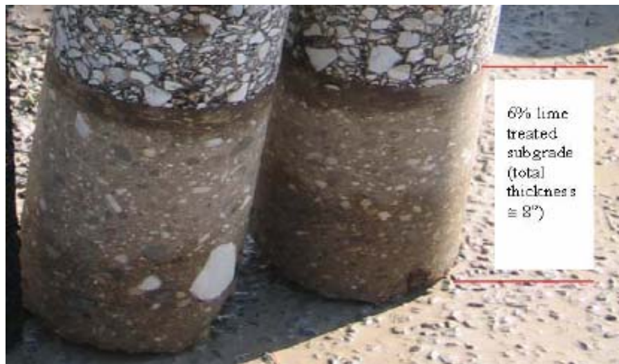
Figure 3-2. Field-Extracted Base Core from SH 114.
