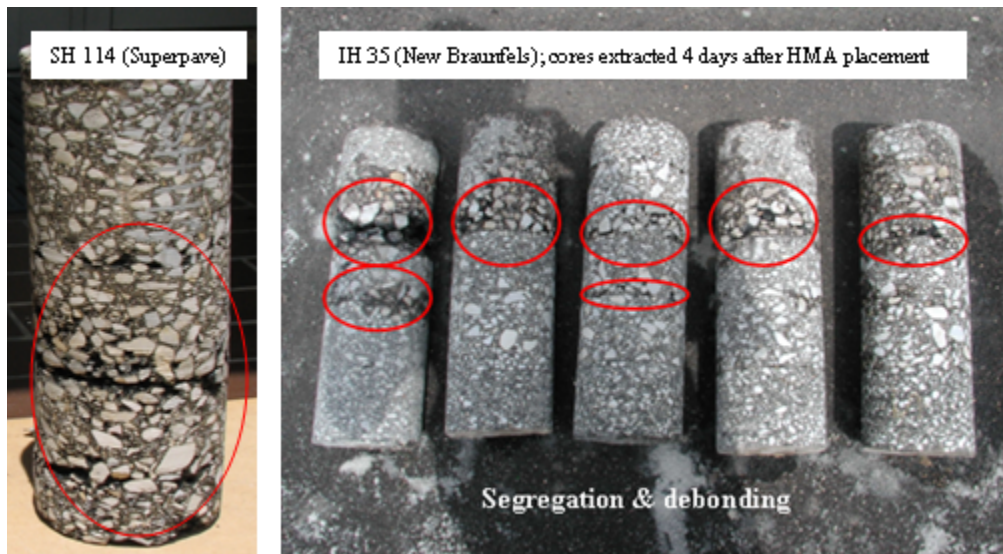
Figure 3-8. Substandard Cores from SH 114 and IH 35.
