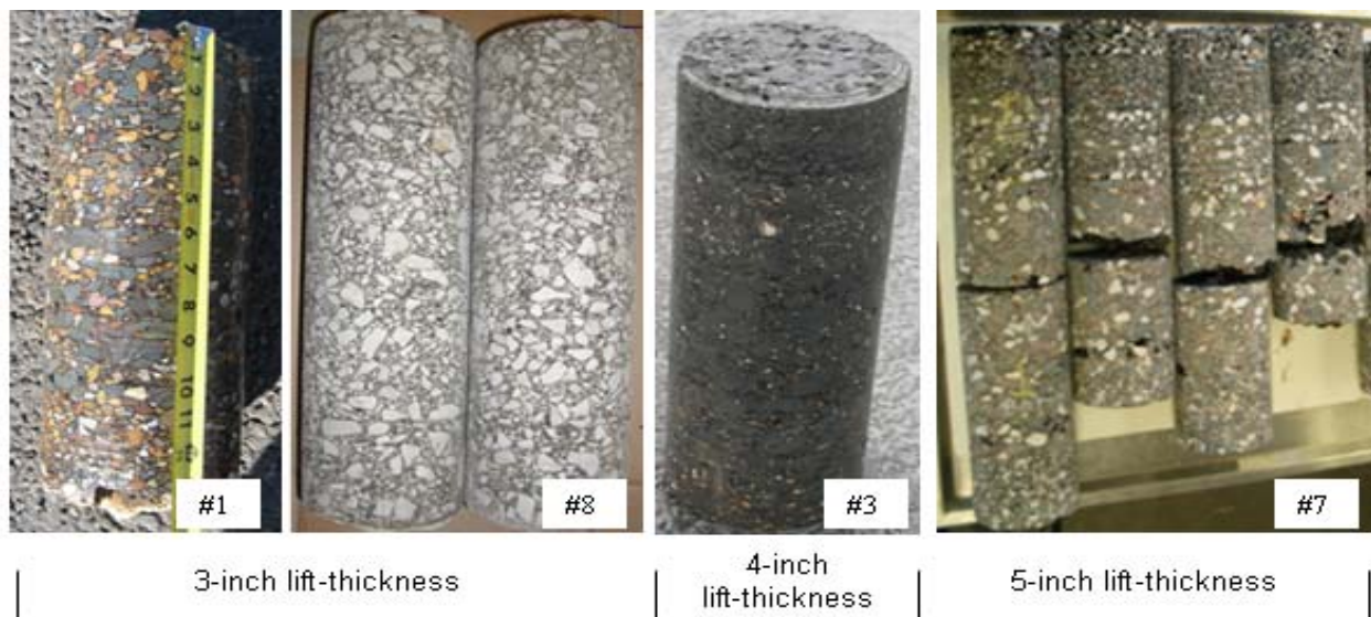
Figure 3-4. Effects of the Compacted Lift Thickness for the 1-inch SFHMA Layer.
