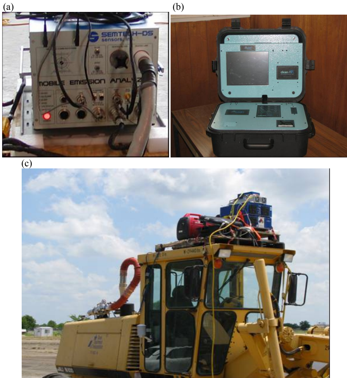
Figure 16. Emission Measurement Instruments: (a) SEMTECH-DS Unit, (b) Axion Unit, and (c) Both Units along with EFM Installed on a TxDOT Grader.
