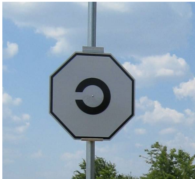
Figure 19. Example of a Test Sign with a Landolt C
