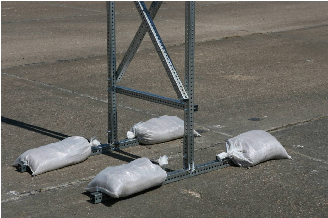
Figure 2. Dual-Support Temporary Sign Support System before Test 463849-1.
