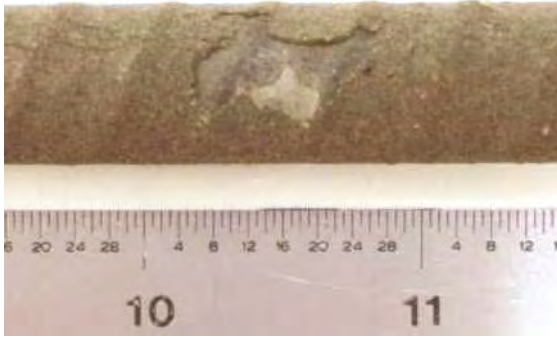
(a) A 50/50 enamel-coated specimen
