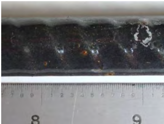
(a) "Minor" signs of corrosion
