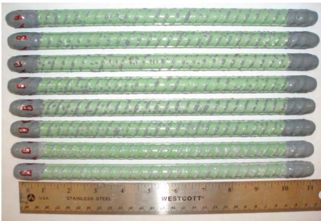
Figure A - 23: Backside of the deformed epoxy-coated salt spray specimens after testing.
