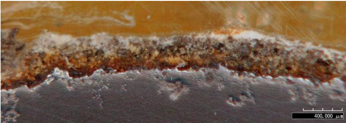
(c) Color gradient within and along a corroded section
