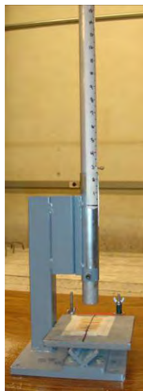
Figure 6.21 Impact test apparatus.
