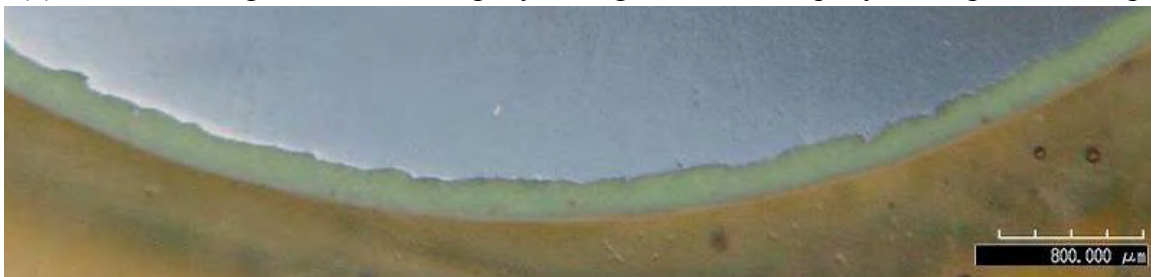
(c) Typical cross-sectional view of an epoxy-coated smooth bar after testing
