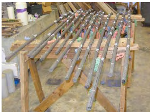
(a) Strain gauges on main reinforcement
