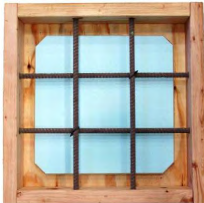
Figure 6.34 Formwork and rebar detail.
