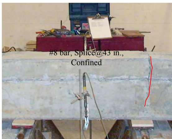
(k) Flexural failure of B-8-3
