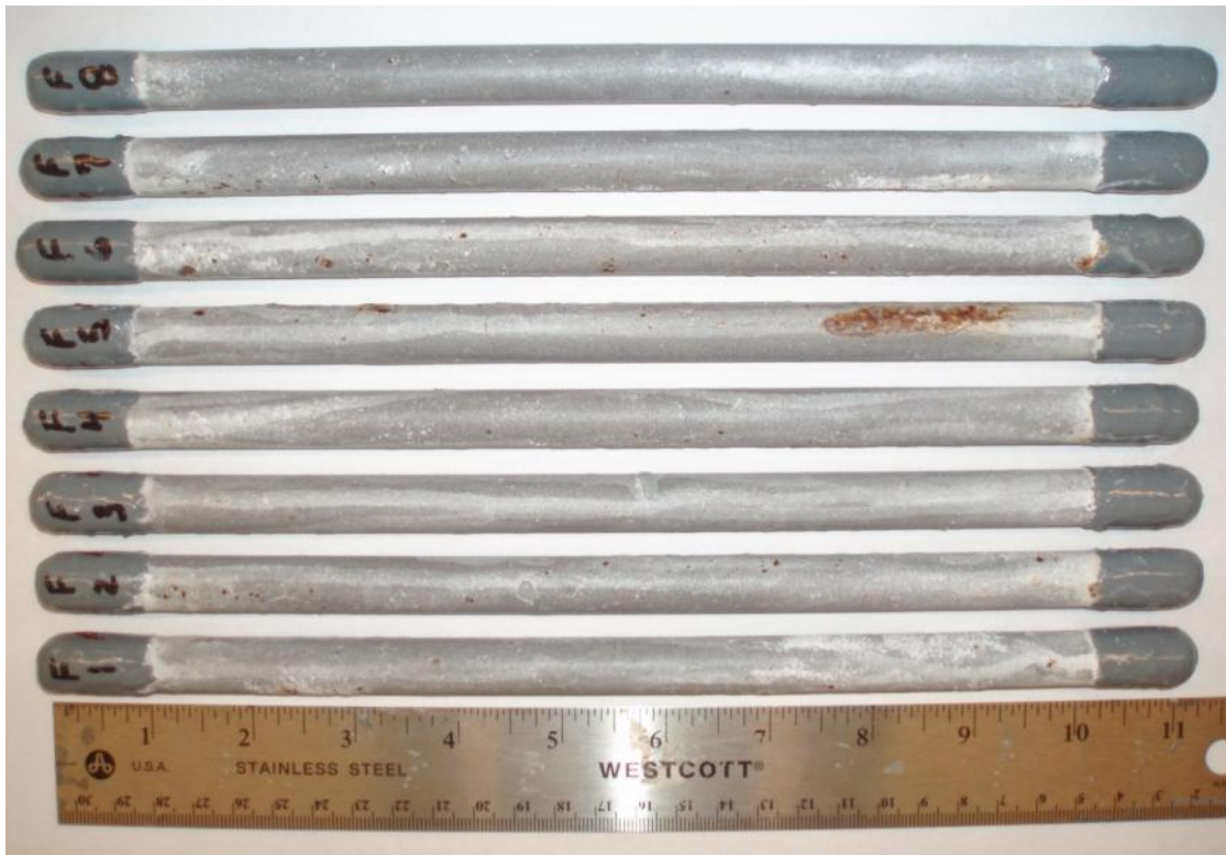
Figure A - 2: Front side of the smooth 50/50 enamel-coated salt spray specimens after testing.
