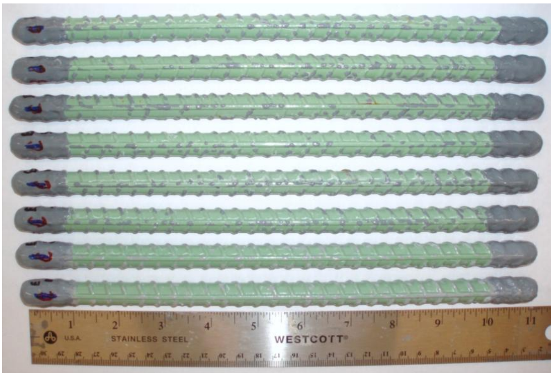
Figure A - 25: Left side of the deformed epoxy-coated salt spray specimens after testing.
