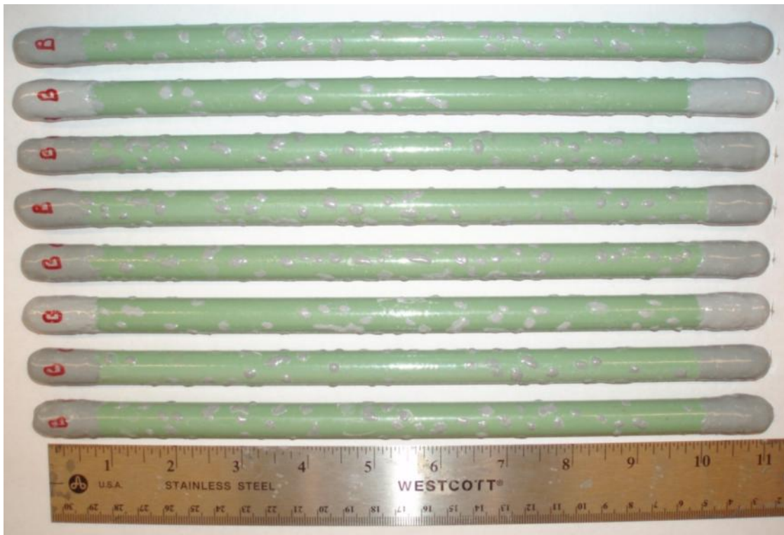
Figure A - 21: Backside of the smooth epoxy-coated salt spray specimens after testing.
