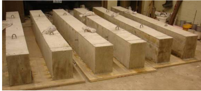
(b) Finished beam specimens
