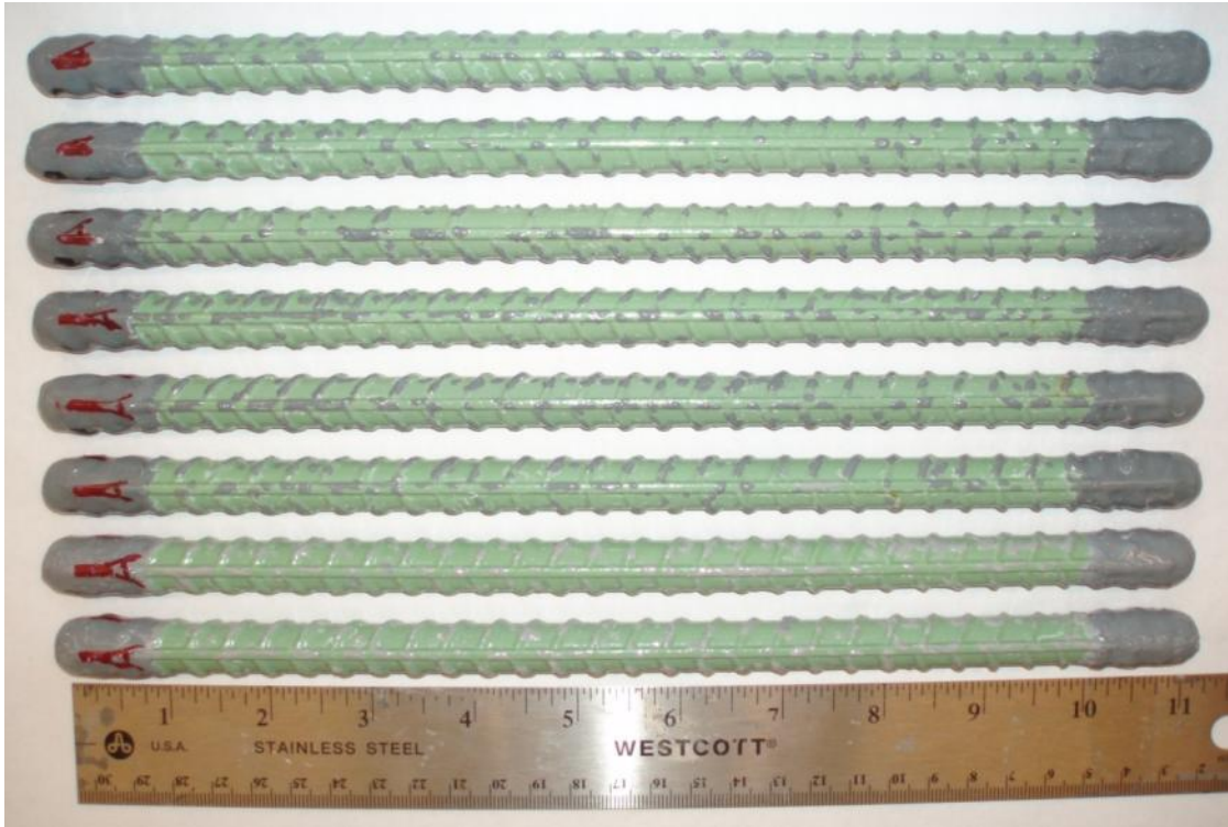
Figure A - 24: Right side of the deformed epoxy-coated salt spray specimens after testing.
