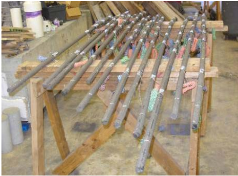
(a) Strain gauges on main reinforcement
