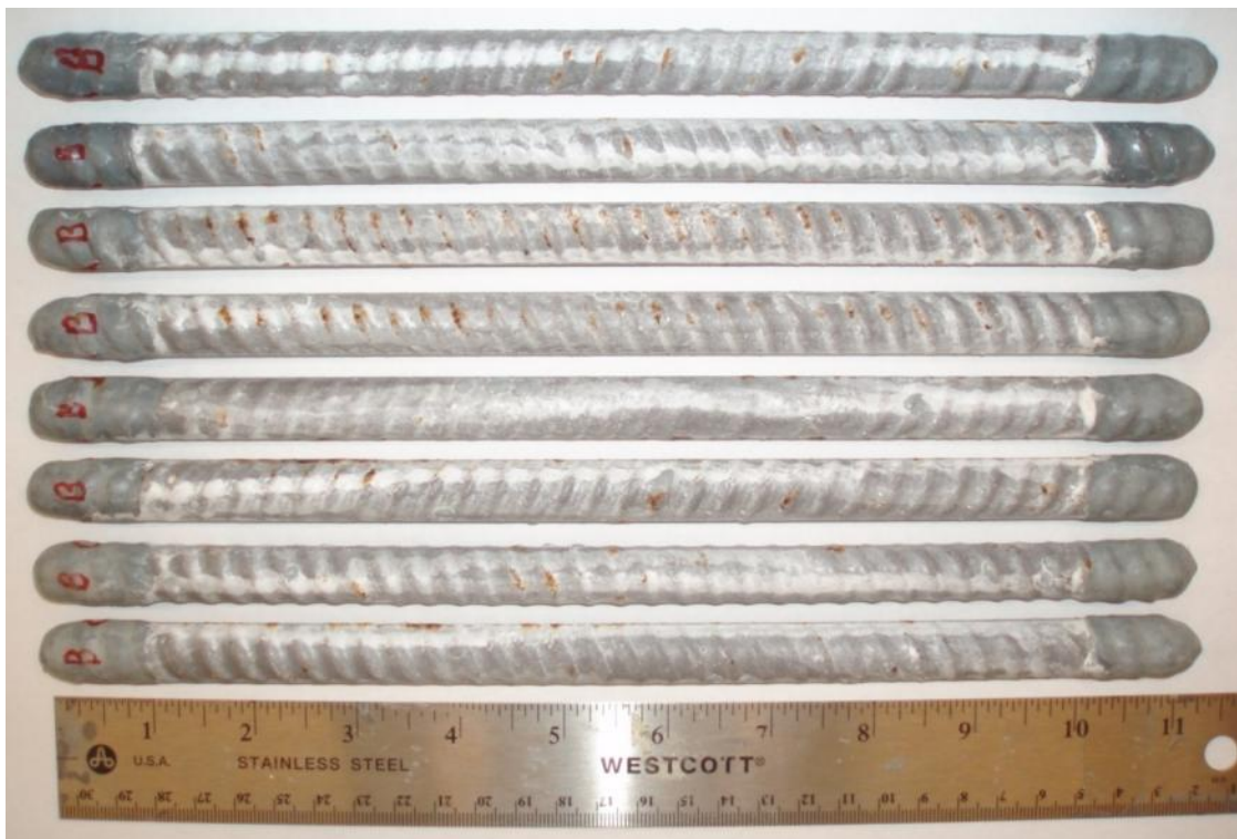
Figure A - 5: Backside of the deformed 50/50 enamel-coated salt spray specimens after testing.
