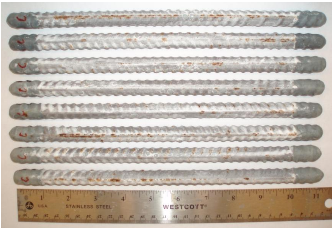
Figure A - 7: Left side of the deformed 50/50 enamel-coated salt spray specimens after testing.
