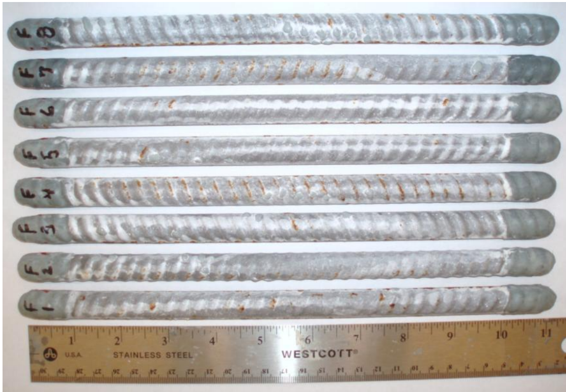
Figure A - 4: Front side of the deformed 50/50 enamel-coated salt spray specimens after testing.
