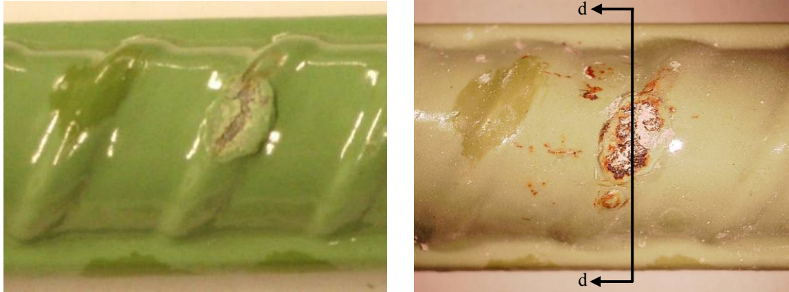
(b) Detailed view of local damage (pre-test) and corrosion around the damage area (post-test)
