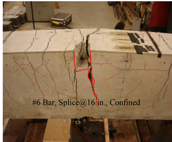
(b) Flexural failure of B-6-2
