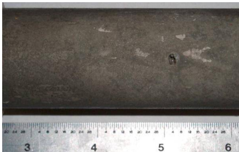
Figure 6.19 A void detrimental to the specimen's performance in the ACT test.
