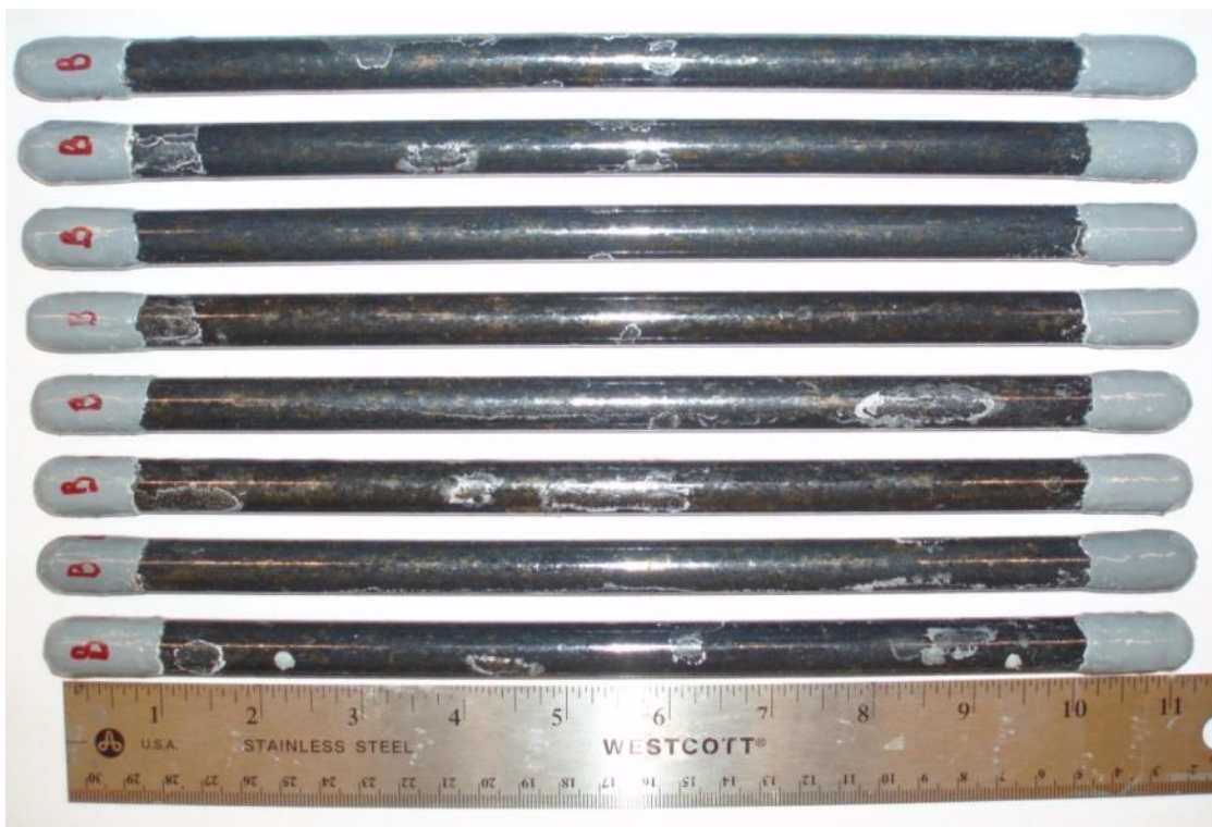
Figure A - 15: Backside of the smooth pure enamel-coated salt spray specimens after testing.
