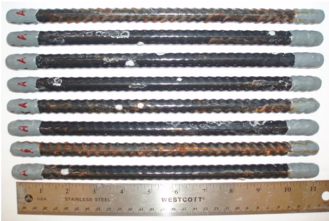
Figure A - 18: Right side of the deformed pure enamel-coated salt spray specimens after testing.
