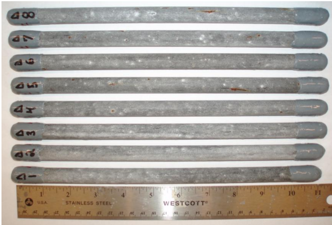
Figure A - 8: Front side of the smooth double enamel-coated salt spray specimens after testing.
