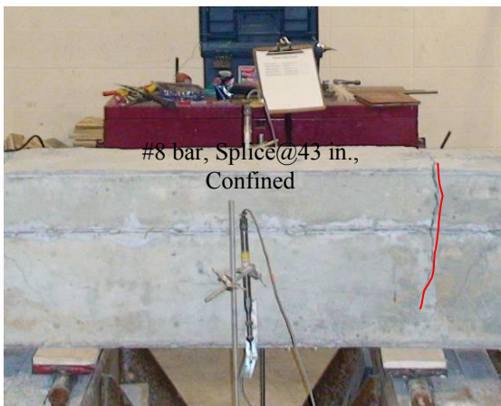
(k) Flexural failure of B-8-3
