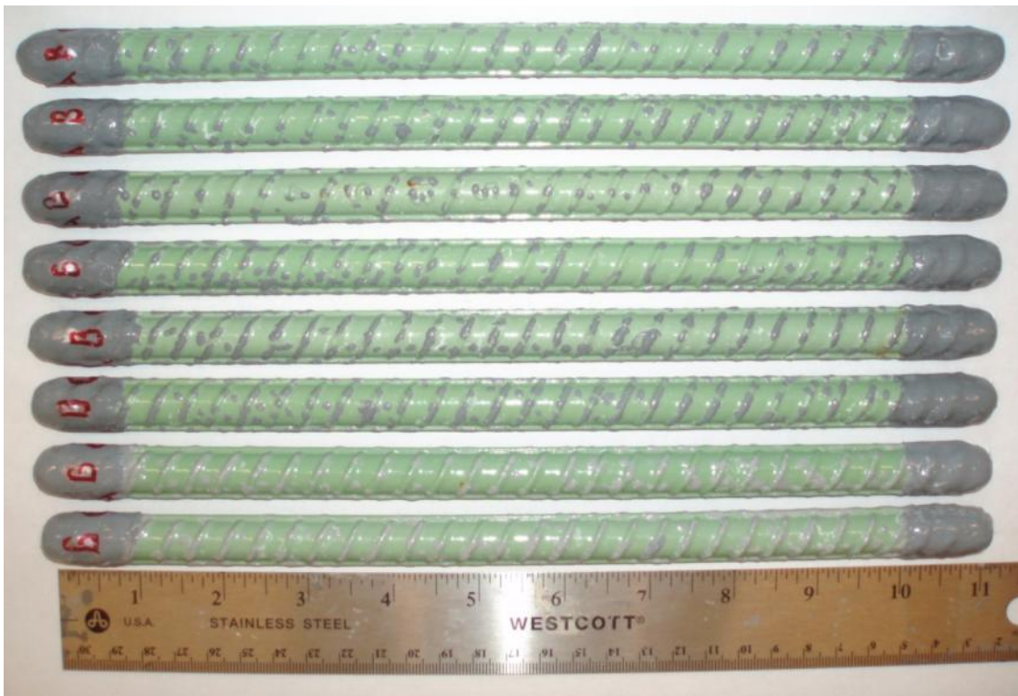
Figure A - 23: Backside of the deformed epoxy-coated salt spray specimens after testing.
