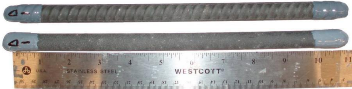
Figure 6.2 Typical smooth and deformed salt spray specimen prior to testing.
