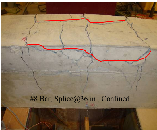
(e) Split failure of B-8-1 with steel yielding
