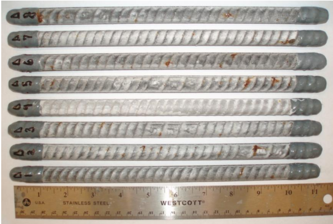
Figure A - 10: Front side of the deformed double enamel-coated salt spray specimens after testing.
