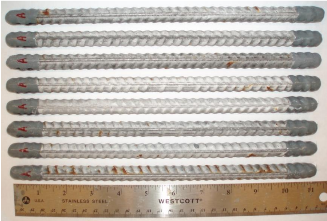
Figure A - 12: Right side of the deformed double enamel-coated salt spray specimens after testing.
