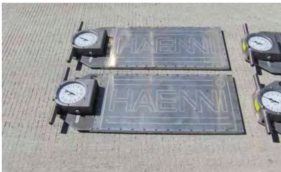
Figure 5.10: TxDOT's portable scales
