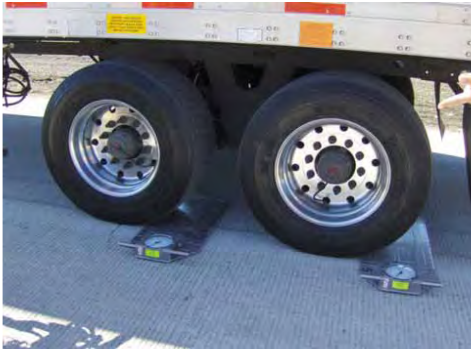
Figure 5.12: Truck leaving scales after weighing two axles
