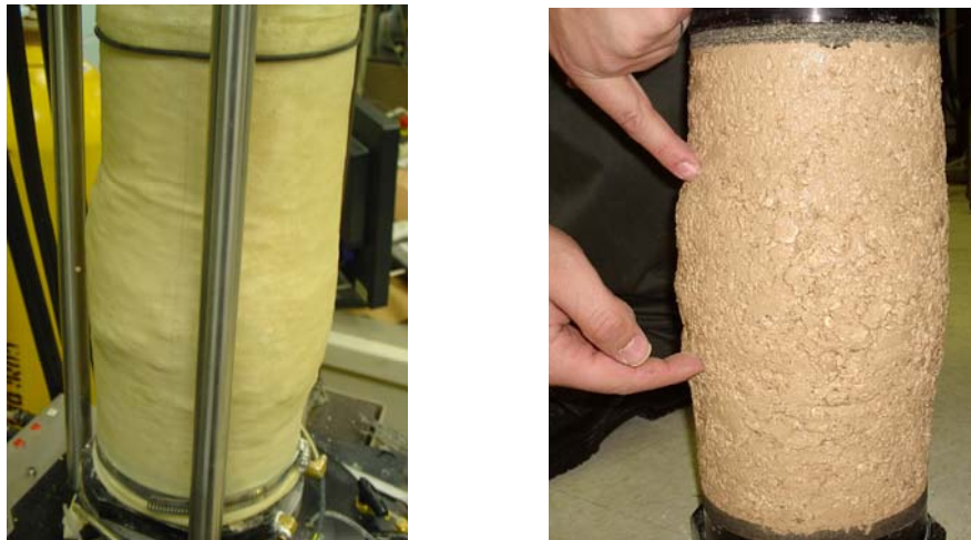
Figure 17 Picture for samples reinforced with two geogrid layers
