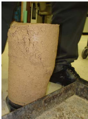
Figure 15 Picture for samples reinforced at mid height
