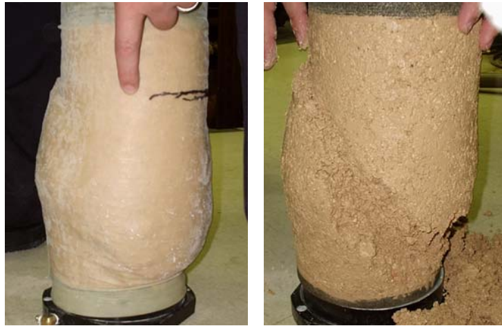
Figure 16 Picture for samples reinforced at upper one-third
