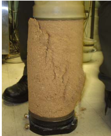
Figure 14 Unreinforced crushed limestone II sample after the end of triaxial compression test
