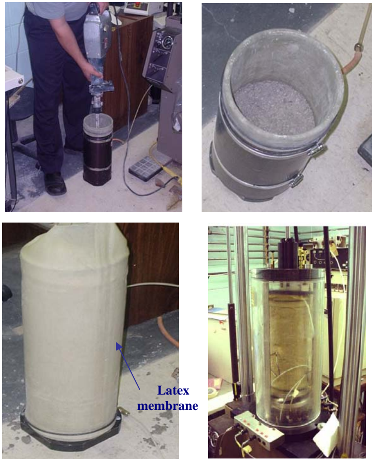
Figure 6 Preparation and testing of crushed limestone sample
