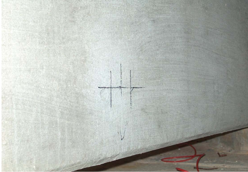
Figure 189 Initial marking on the continuity diaphragm for placing transducer
