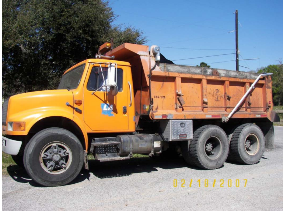
Figure 7 Test truck of GVW 48.66 kips used at site
