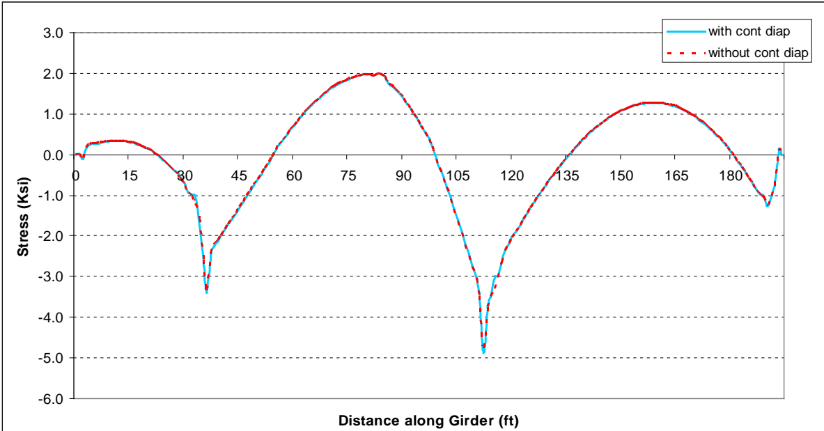
Figure 38 Comparison of stresses of Case I and Case III for bottom elements in Girder 1
