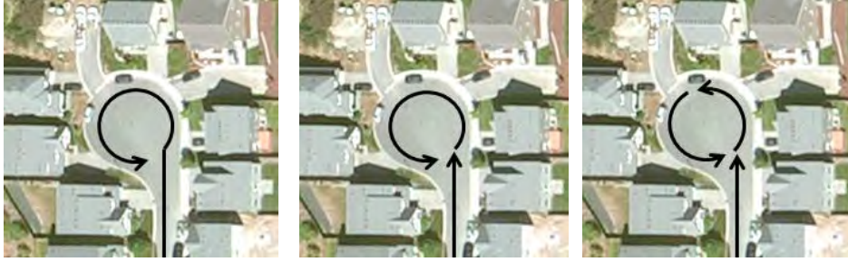
Figure 8.1: Types of Cul-de-Sac Street Segments. Cul-de-sac were commonly represented by one (left), two (middle), or three (right) street segments.
