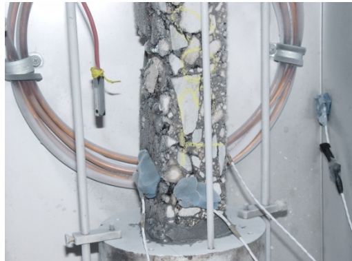
Figure 47. Failed 302 mix specimens after TSRST.
