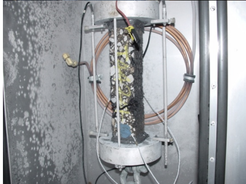
Figure 46. Failed 442 mix specimens after TSRST.
