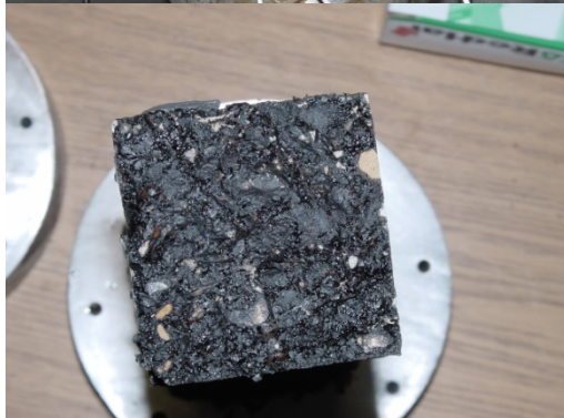
Figure 48. Failed FRL mix specimens after TSRST.
