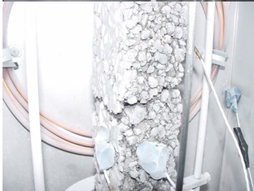
Figure 49. Failed SMA mix specimens after TSRST.
