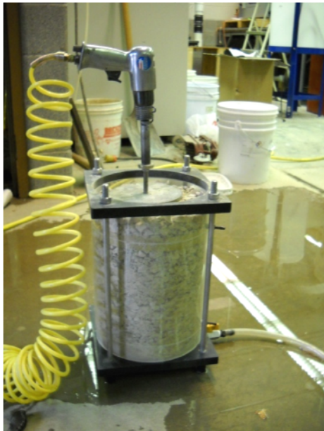
Figure 19. Permeameter with compacted aggregate subbase and vibrating tamper.
