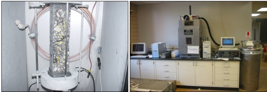
Figure 41. Left: TSRST sample after failure; Right: TSRST System
