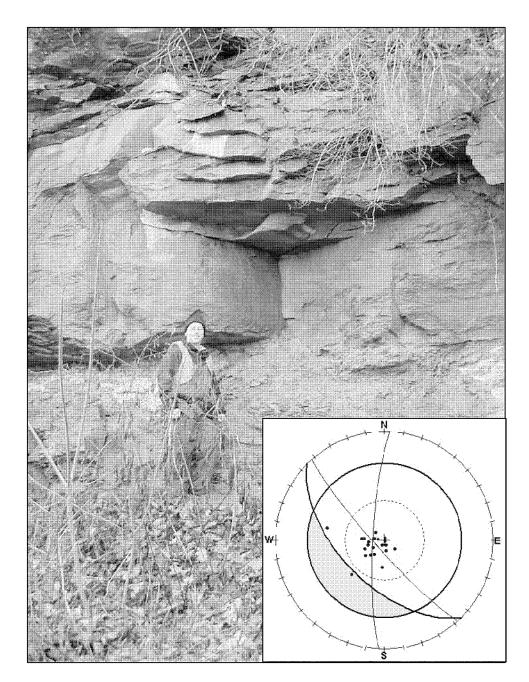
Figure 3.9: Example of a typical road cut, from site designated as WAS-7-39.5, with its associated dip vector stereoplot. Notice that neither plane failures nor wedge failures can be identified through the conventional use of Markland failure criterion as almost all of the dip vectors fall outside the critical zone.
