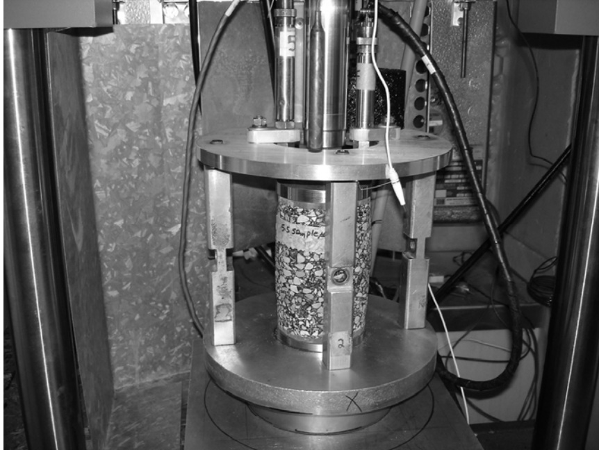
Figure 5.8 Unconfined cyclic compression load test set up
