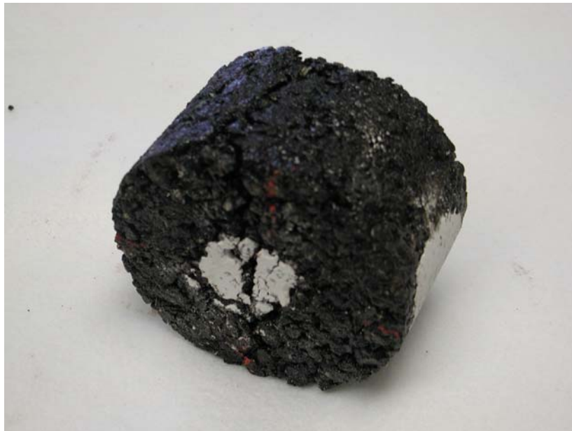
Figure 2.15. Fatigue Cracking in lab Specimen at Intermediate Stages
