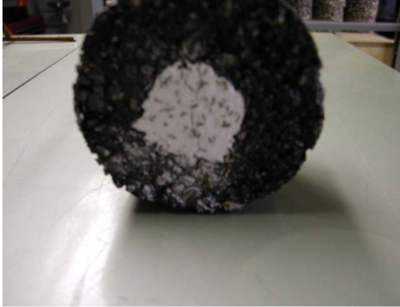
Figure 2.14. Fatigue Cracking in lab Specimen at Early Stages
