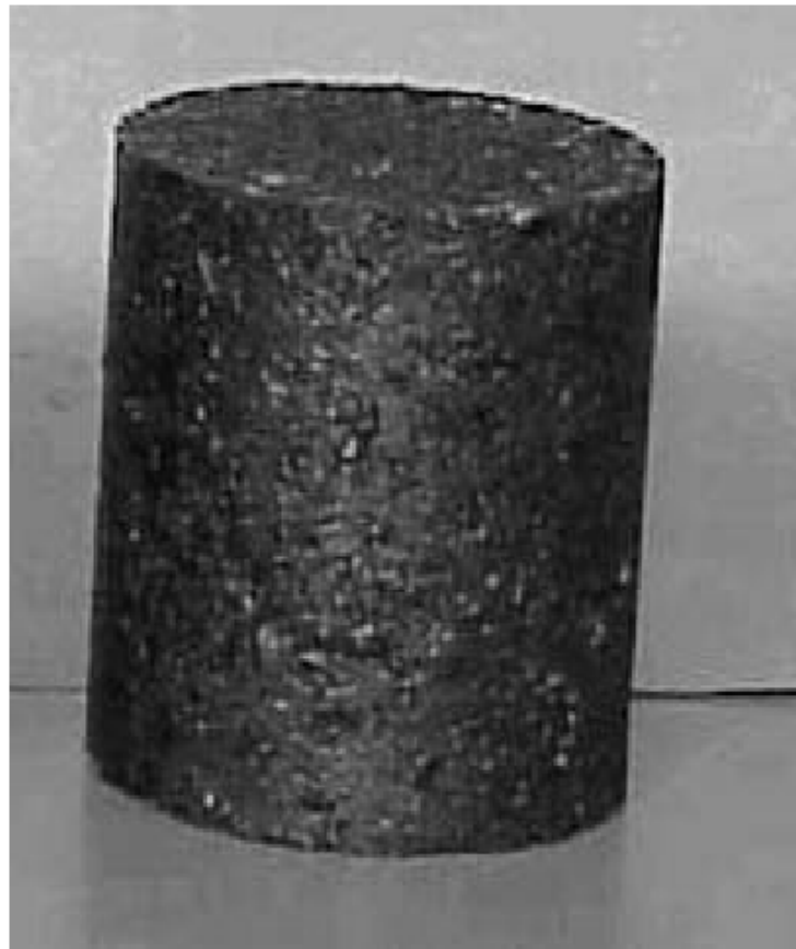
Figure 5.1 Compacted test specimen (6-inch diameter, 7-inch height)
