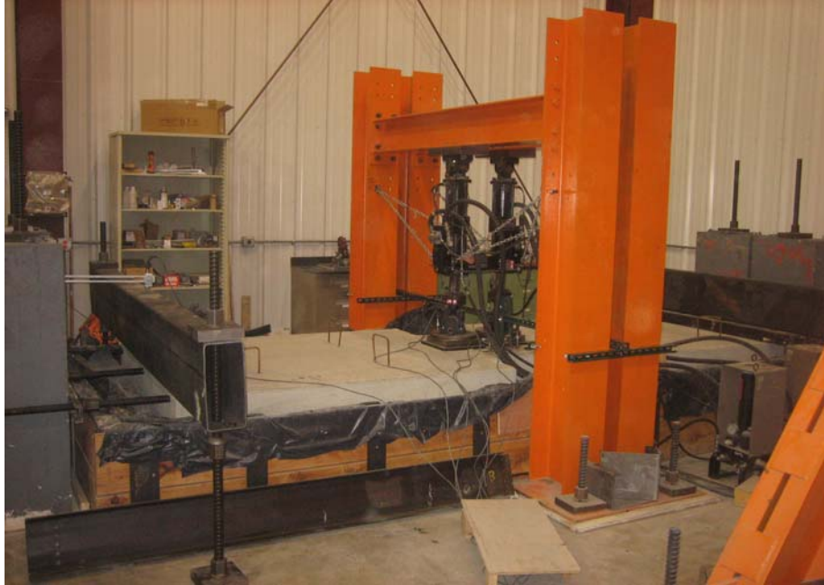
(a) Slab Test set-up
