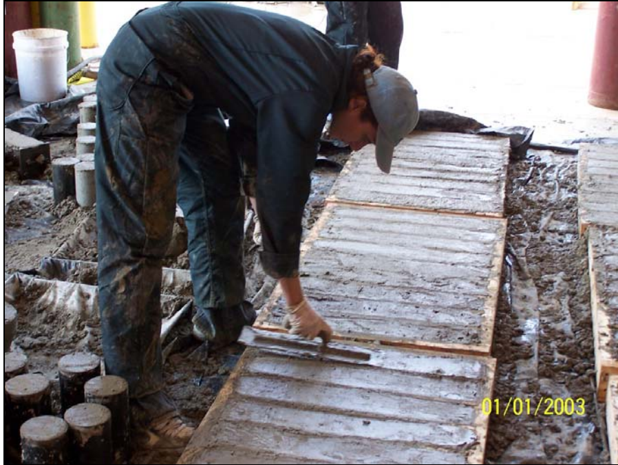
(a) Casting of beams
