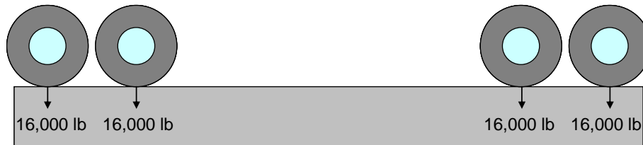
(b) A single axle with single wheels with a tandem axle simulating the front tandem axle
