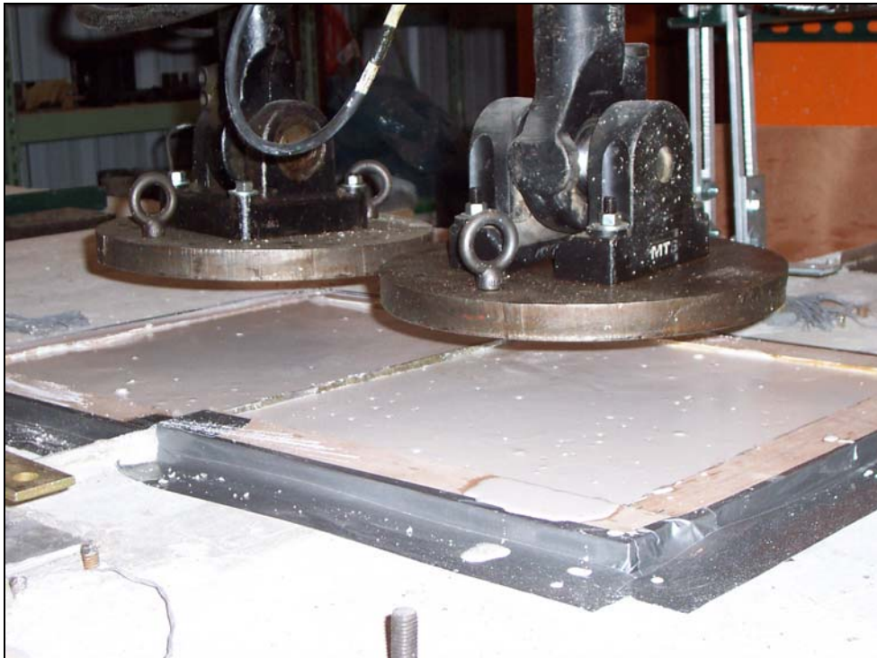
Figure 4.2 Loading Actuator at Slab Joint
