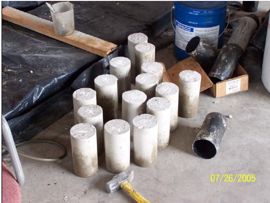
(b) De-molded 4 x 8 inch 15 cylinders
