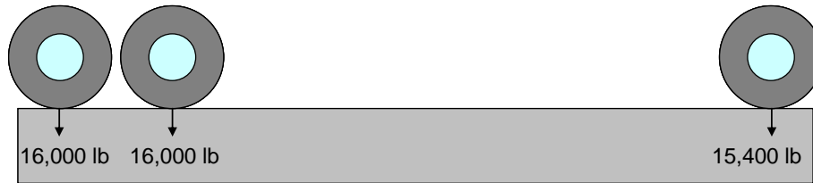
(b) A single axle with single wheels with a tandem axle simulating the front tandem axle
