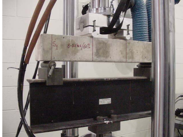
Figure 2.8 Beam Fatigue Fixture with Simple Third-Point Loading
