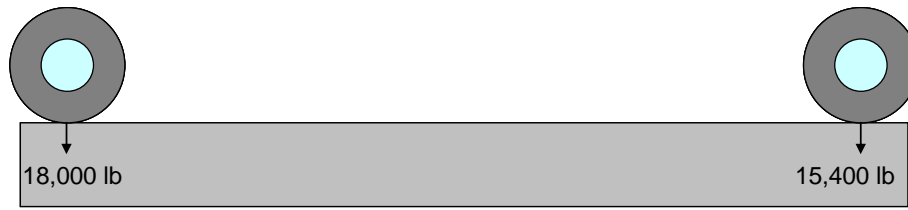
(a) A single steering axle with single wheels and a single drive axle with dual wheels
