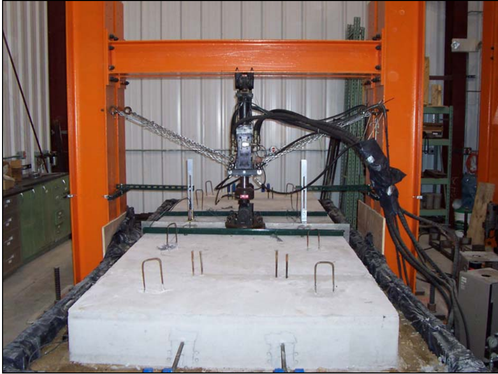
Figure 4.1 Full-Scale Trial Slab with Loading Setup
