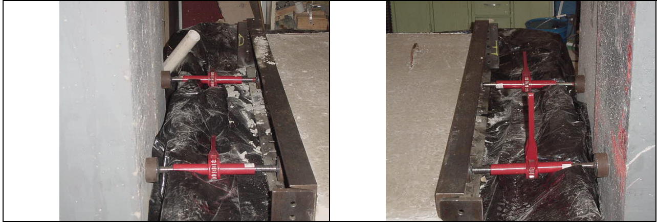
Figure 4.28 Photo of Jacks placed on both sides of the Slab
