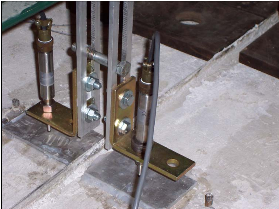
Figure 4.4 LVDTs Across Joint for Measuring Relative Deformation
