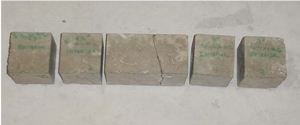
Figure 2.38 Cubes sawed out of failed beams in fatigue test
