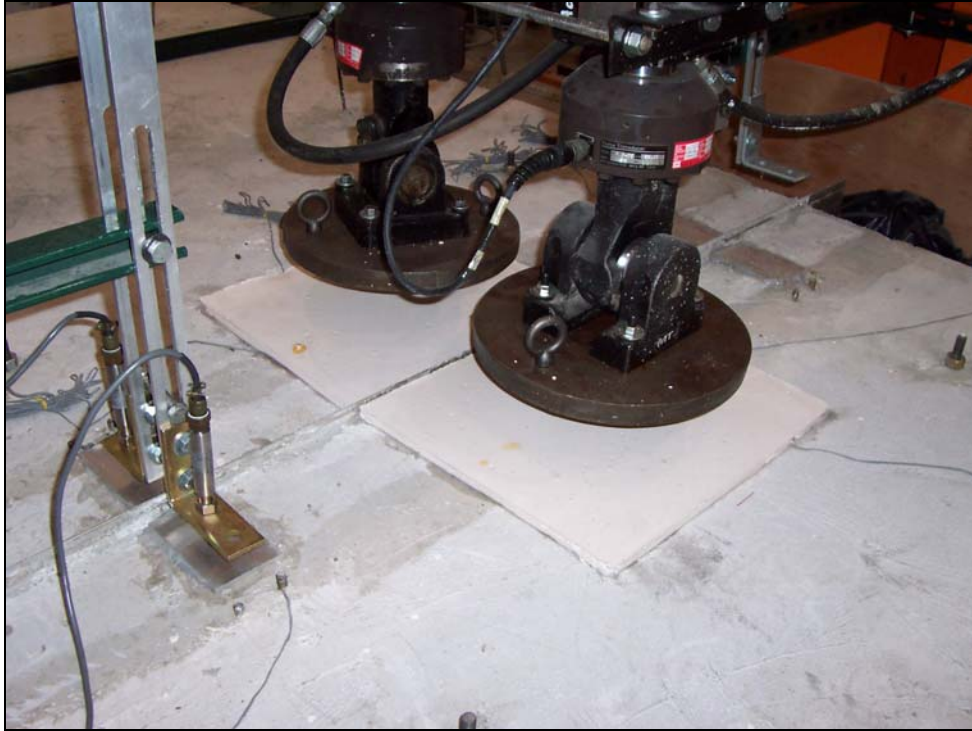
Figure 4.5 Loading and Un-loading Sequence with LVDTs Across Joint
