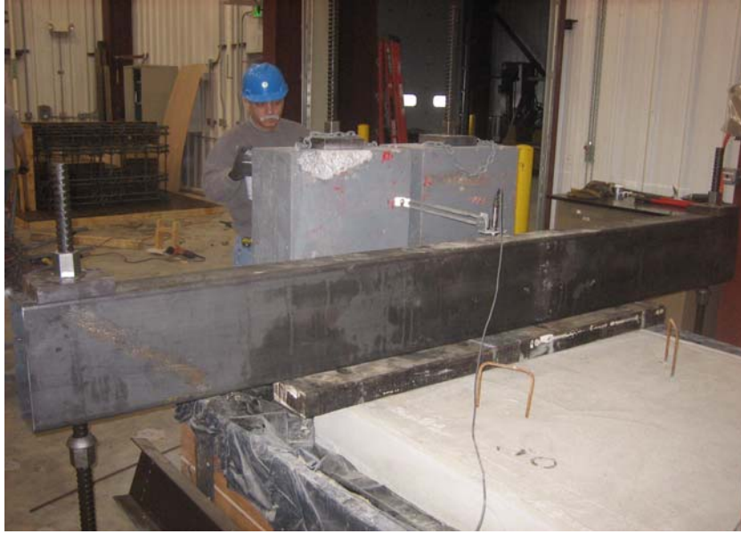
Figure 4.25 Steel Tube (14x6) Placed at the End of the Slab
