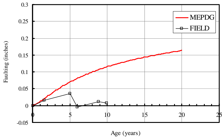
(b) Joint faulting (mm)
