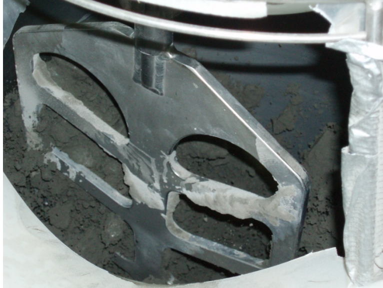
Figure 3-2: Turning Point of UHPC
