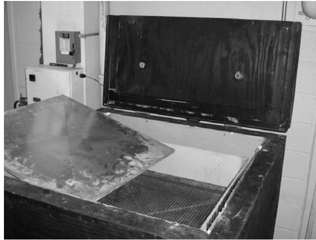
Figure 3-4: Michigan Tech’s UHPC Thermal Treatment Cure Chamber
