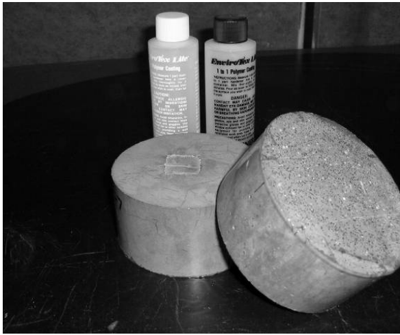
Figure 3-10: Epoxy-coated UHPC Specimens for RCPT
