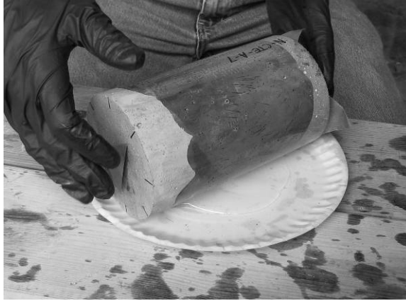
Figure 3-16: Epoxy-coating CTE Specimen
