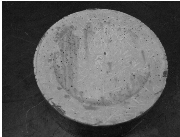
Figure 4-11: Surface Staining of UHPC Specimen after ASTM C 1202 Test
