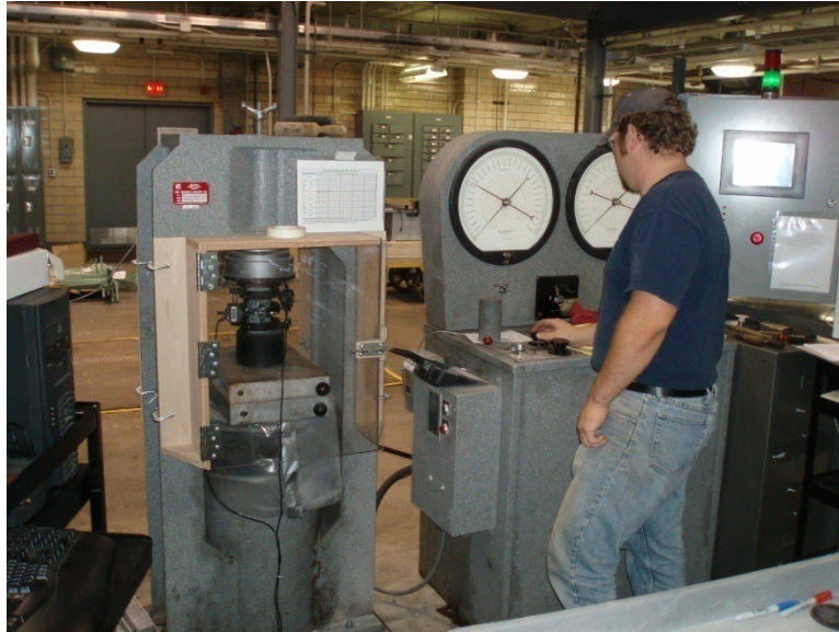
Figure 3-7: Baldwin CT 300 Compression Testing Machine
