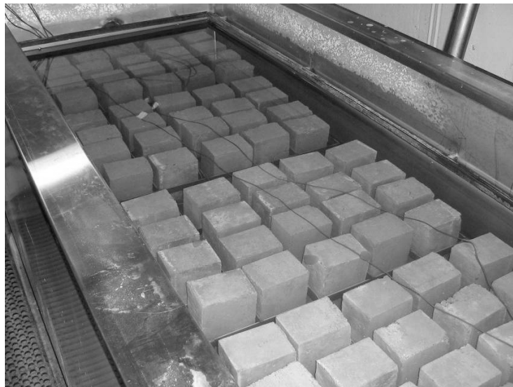
Figure 3-13: MTU 80-specimen Freeze-Thaw Chamber (Procedure B)
