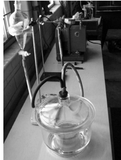
Figure 3-11: ASTM C 1202 Specimen Preparation Setup
