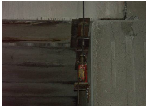
Photo 3-7. Force application using hydraulic jacks at both ends of the beam
