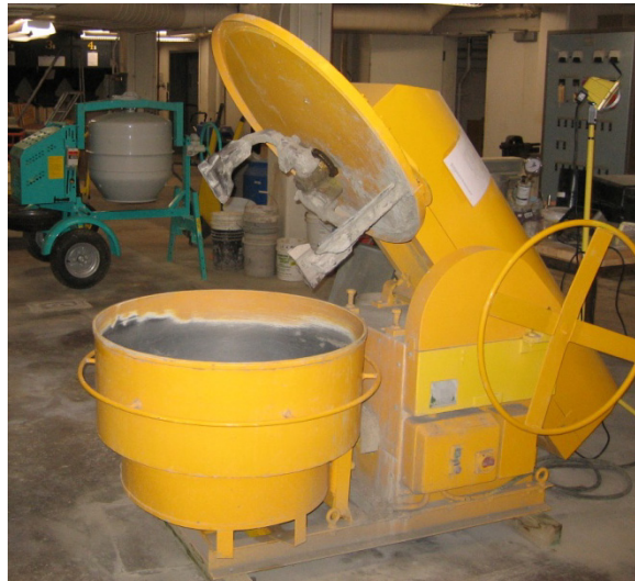
Figure 4-5. Laboratory pan mixer
