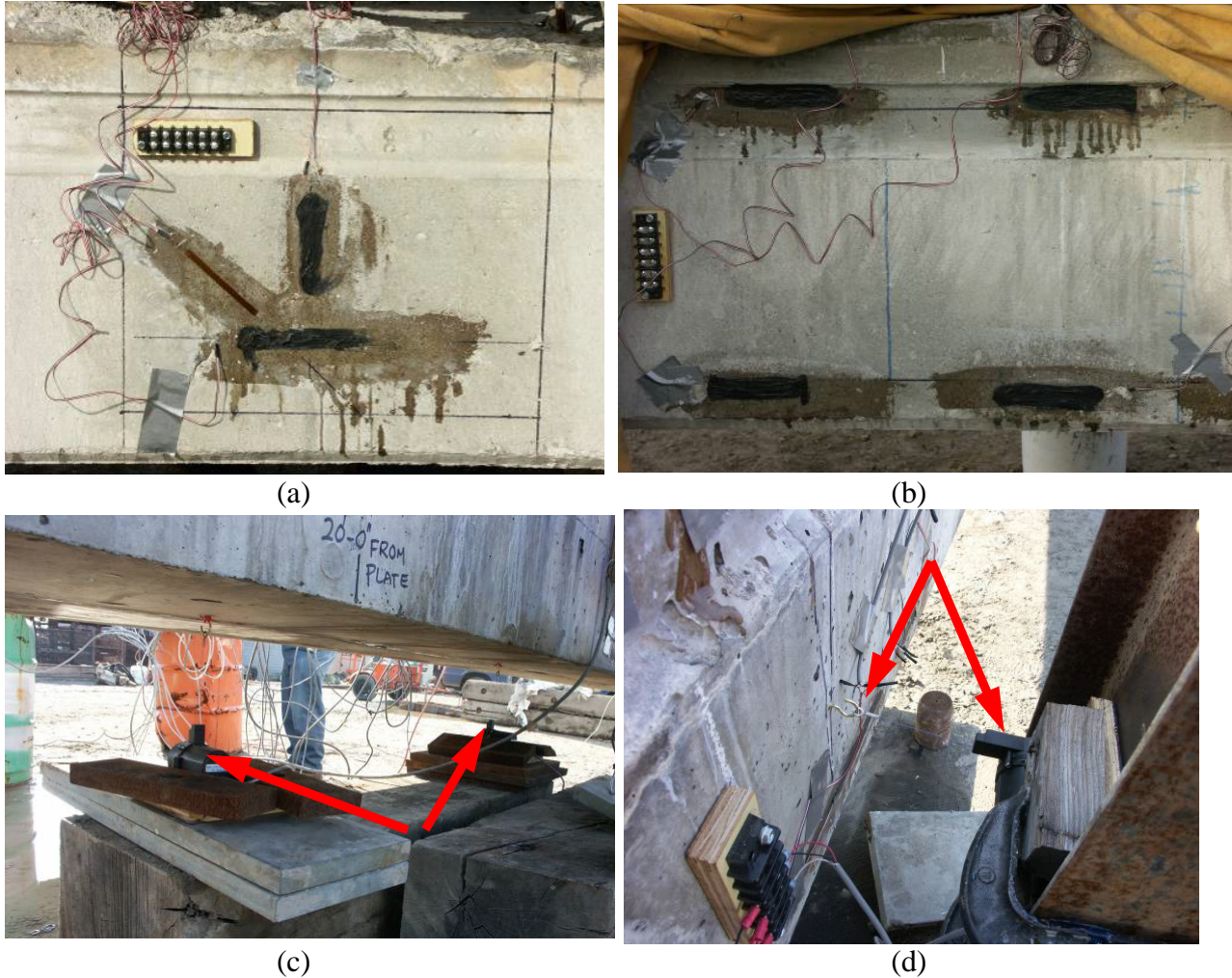
Photo 3-10. Strain gauges at (a) beam end and (b) mid-span and cable actuated position sensors at mid-span for (c) vertical and (d) horizontal displacement measurement.
