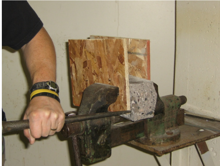
Figure 4-8. Surface preparation of the substrate concrete specimen
