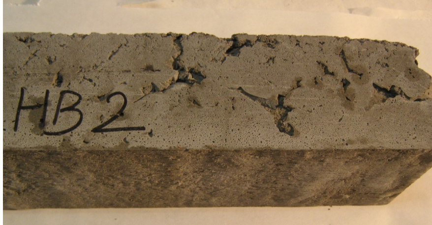
Figure F-16. Photograph of HB2 Repair Mortar Sample Cast for F/T Testing
