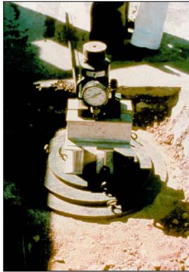
Figure B.5 Photo of plate load testing apparatus (NHI 1998)
