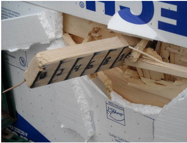
Figure 3.21d Test #53 Post Impact
