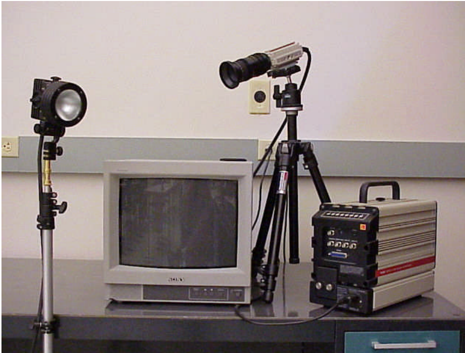
Figure 2.11 Kodak Motion Corder Analyzer PS-110 (Alciatore)
