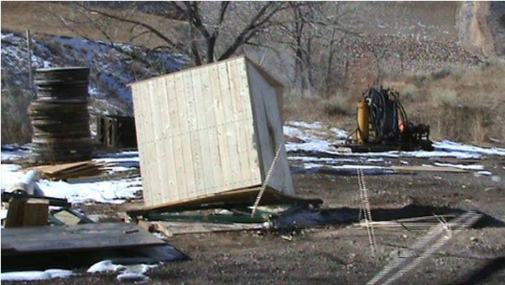
Figure 3.6c Test #37 Video Still of Front Vertex Uplift
