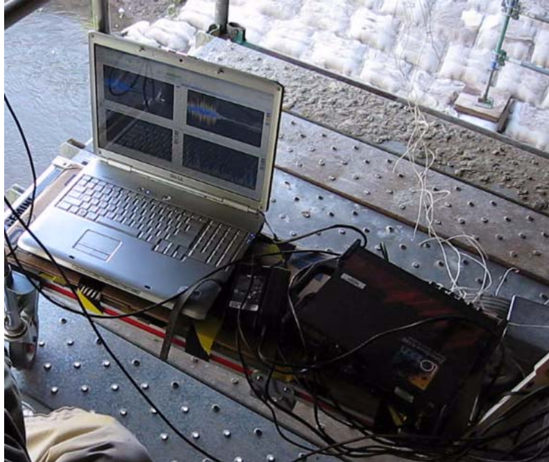
Figure 4.3 Typical field operational vibration test setup
