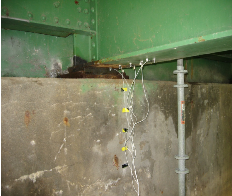
Figure 4.25 Operational vibration response measurement of a beam near the boundary condition
