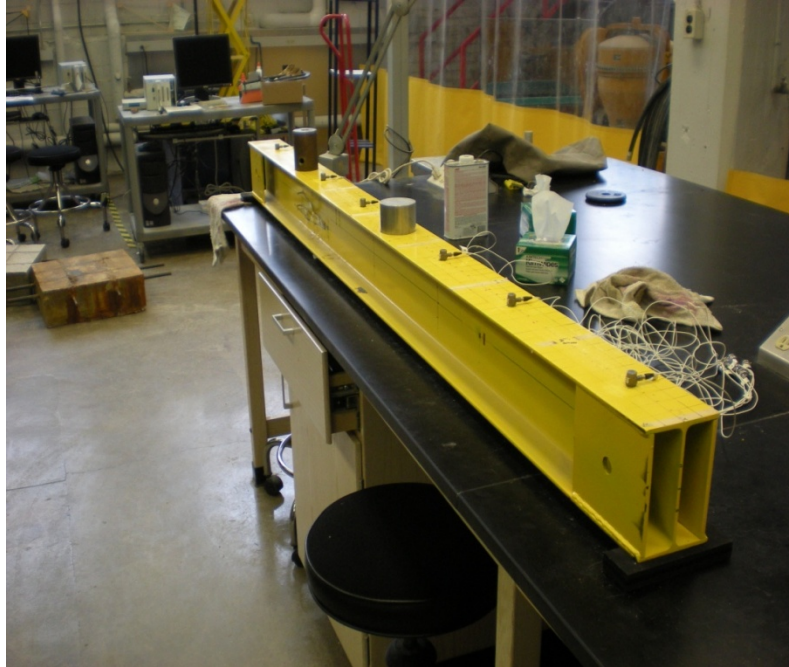
Figure 3.3 Typical laboratory I-beam setup with six fixed accelerometers and two damage zones
