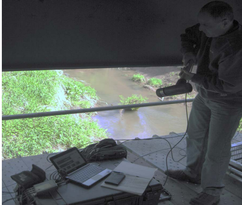
Figure 4.15 Data acquisition system setup with large impact hammer used to excite each beam
