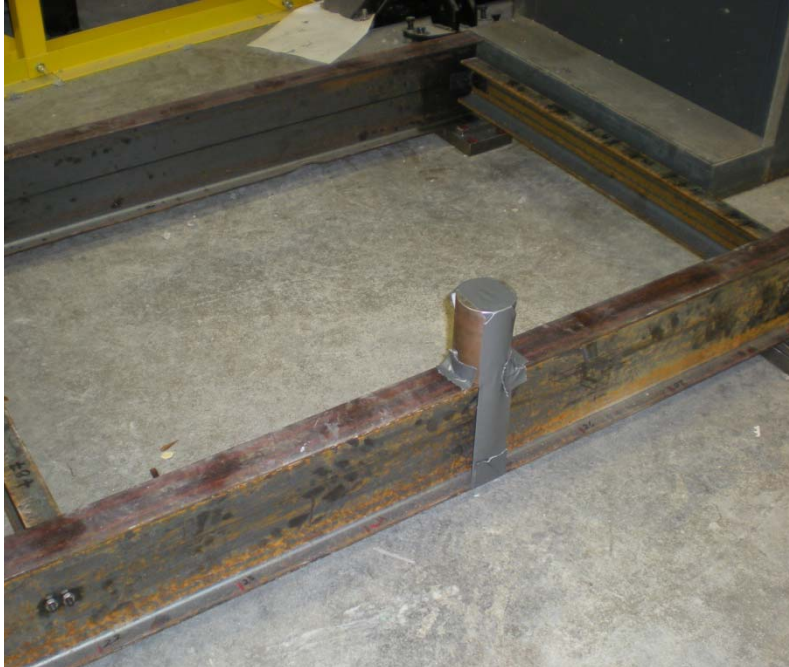
Figure 3.27 Mass (1500 g) added to top flange of beam 1, 20 inches from the far end
