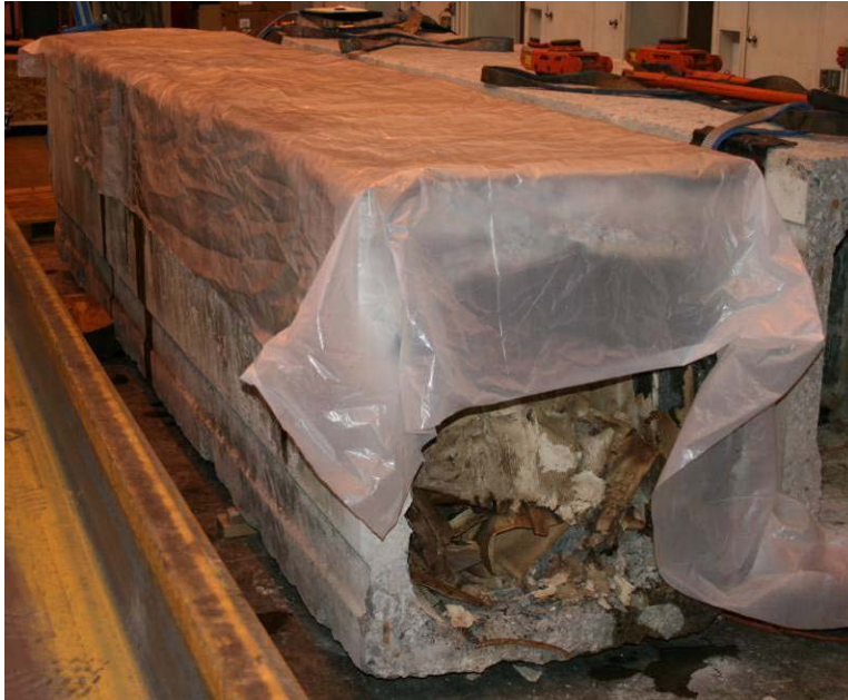
Figure 6-5: Plastic Tarp Covering the Beam During the Moistening Procedure
