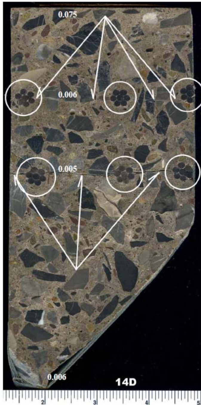
Figure 4-12: Petrographic Examination of Core 14D from Beam CC3
