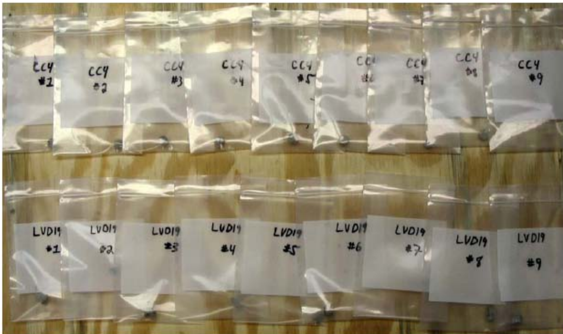
Figure 4-9: 5/8 inch Diameter Plugs Submitted for Chloride Analyses
