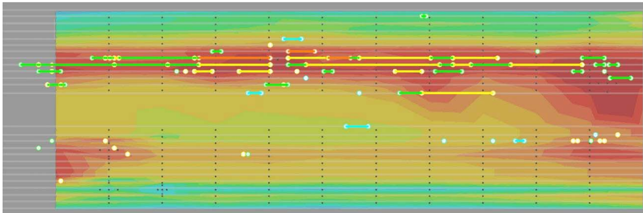
Figure 7-7: Overlay of Damage Profile on Half Cell Potential Map for Beam LV19
