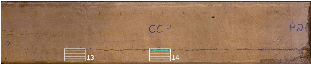
Figure 5-12: Location of 2 nd Layer Punch outs on Beam CC4
