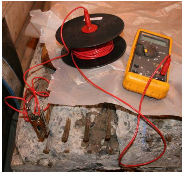
Figure 6-3: Electrical Connection between Multi-meter and Strand.
