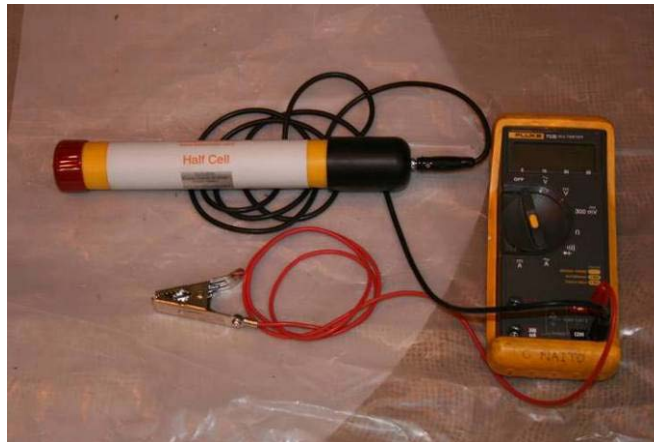
Figure 6-1: Half-Cell Electrode with Multimeter
