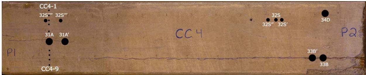
Figure 4-2: Core Locations for Beam CC4
