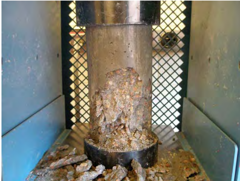
Figure 7.5 Photograph of Compressive Strength Failure (ASTM C 39, AASHTO T 22)
