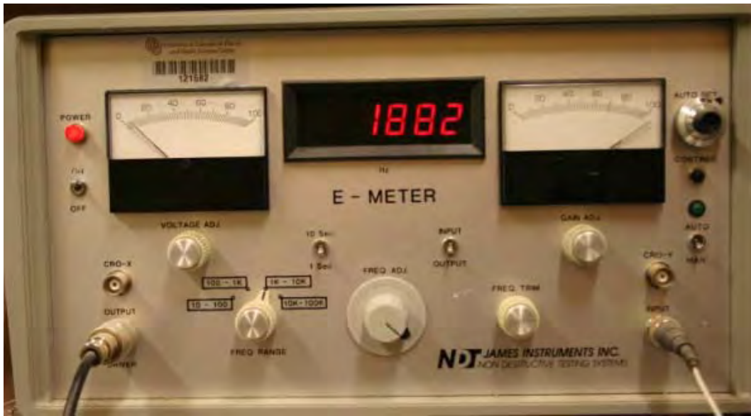
Figure 7.30 Photograph of Durability Testing Apparatus (ASTM C 666, Procedure A)
