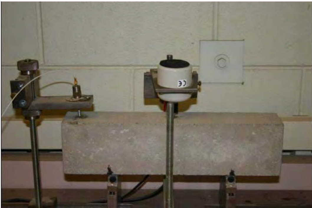
Figure 7.30 Photograph of Durability Testing Apparatus (ASTM C 666, Procedure A)
