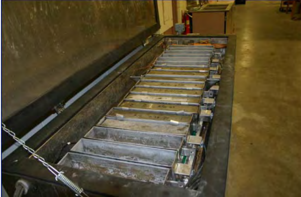
Figure 7.29 Photograph of Freeze/Thaw Chamber (ASTM C 666, Procedure A)
