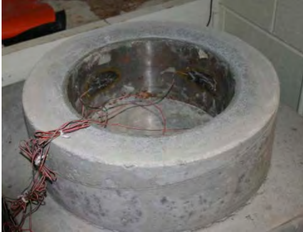
Figure 7.38 Photograph of Restrained Ring Shrinkage Specimen (ASTM C 1581, AASHTO PP34)
