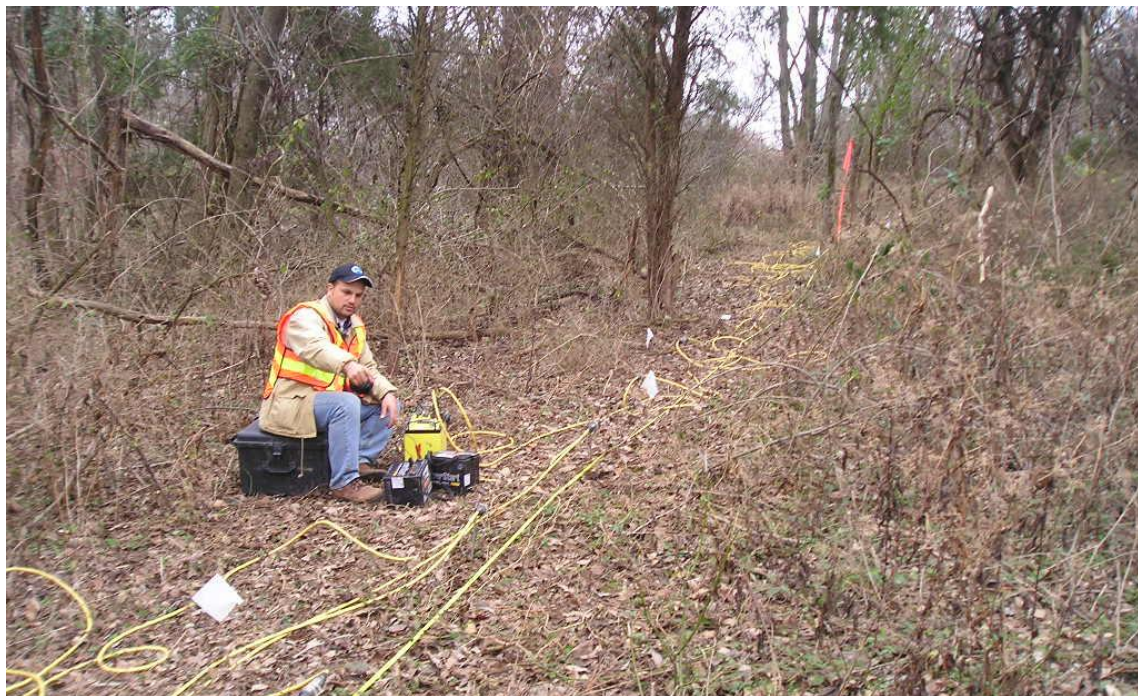
Figure 3: Electrical resistivity data were acquired using a SuperSting R8 resistivity unit equipped with 40 electrodes.
