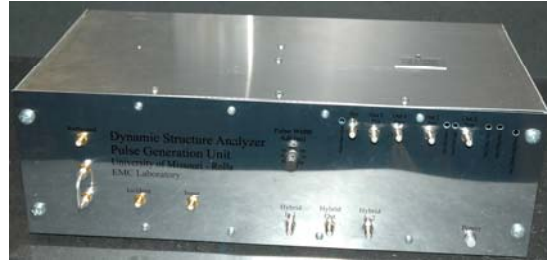
(b) Fast ETDR instrument
