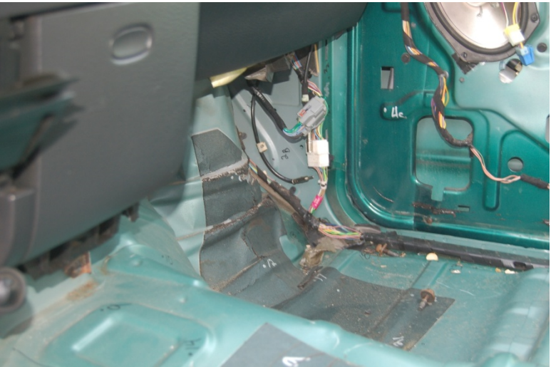
Figure 35. Occupant Compartment Deformation, Test No. NYTCB-5
