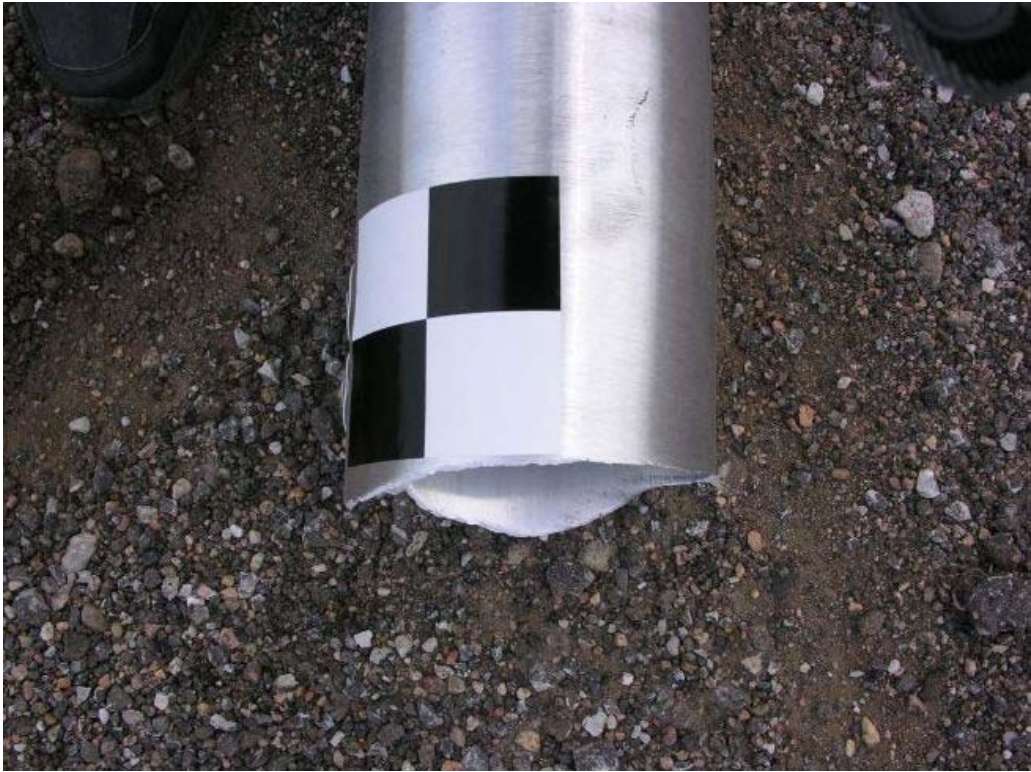
Figure 36. System Damage - Upper Portion of Pole, Test NYPP-1
