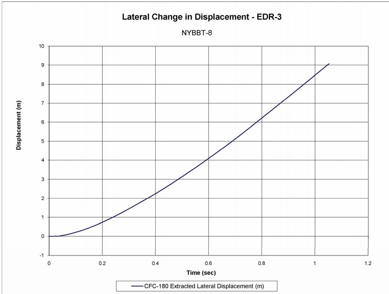
Figure U-6. Graph of Lateral Occupant Displacement (EDR-3), Test No. NYBBT-8
