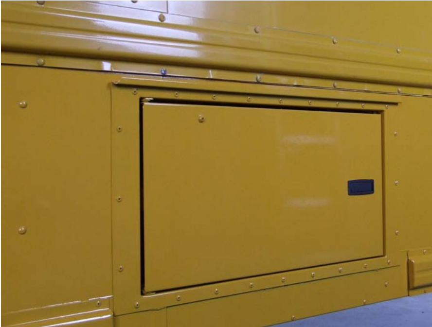
Figure 8 -Typical battery box style enclosure installed in a late model IC conventional school bus body
