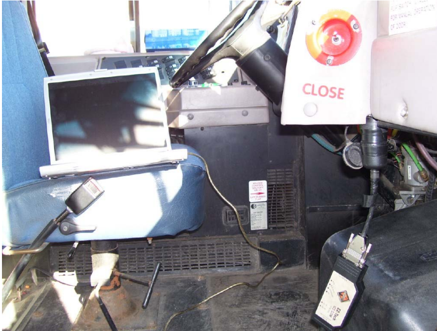
Figure 16 - J1939 Vehicle Data Bus Interface and Laptop
