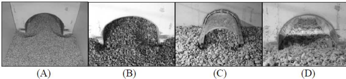
Figure 2-16 Examples of scour at entrance of culvert for 7-mm gravel (A), 16-mm angular gravel (B), 35-mm cobbles (C), and 37-mm angular rock (D)
