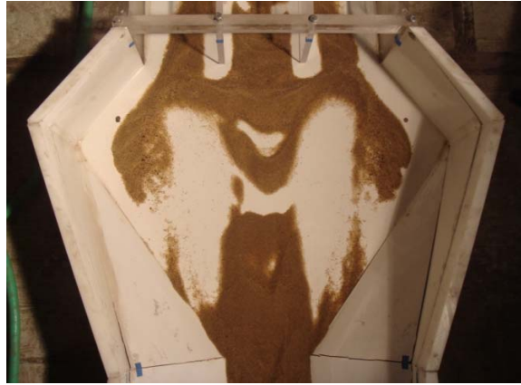
Figure 3-37 Sediment deposition pattern upstream the culvert after Test 4
