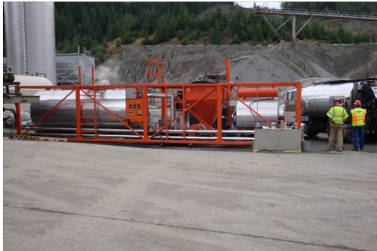
Figure 4. High-shear high speed blender used to add crumb rubber to the PG64-22 asphalt.
