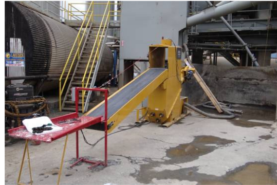
Figure 7. Equipment for introducing fibers into asphalt plant.
