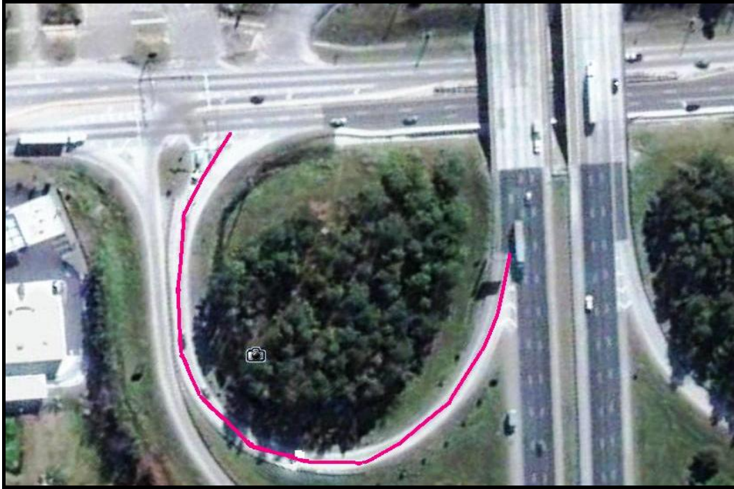
Figure 5.5-C. Free-flow Loop Exit Ramp Segment Length
