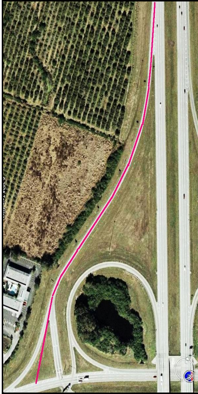
Figure 5.5-B. Out Connection Exit Ramp Length
