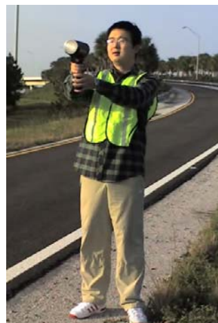
(f) Use of Radar Gun in Data Collection
