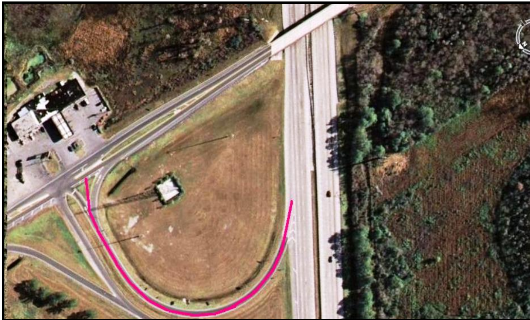
Figure 5.5-D. Parclo Loop Exit Ramp Segment Length
