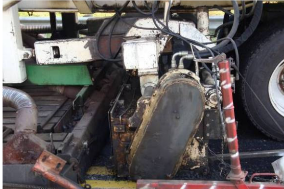
Figure 6. Milling head on left side of unit A removes a five-foot strip from the left side of the lane. An identical milling head removes the same amount from the right side.
