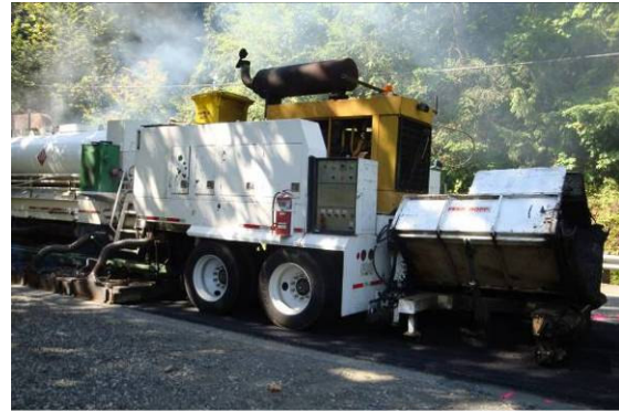
Figure 9. Right front of unit B showing hopper for admixture.
