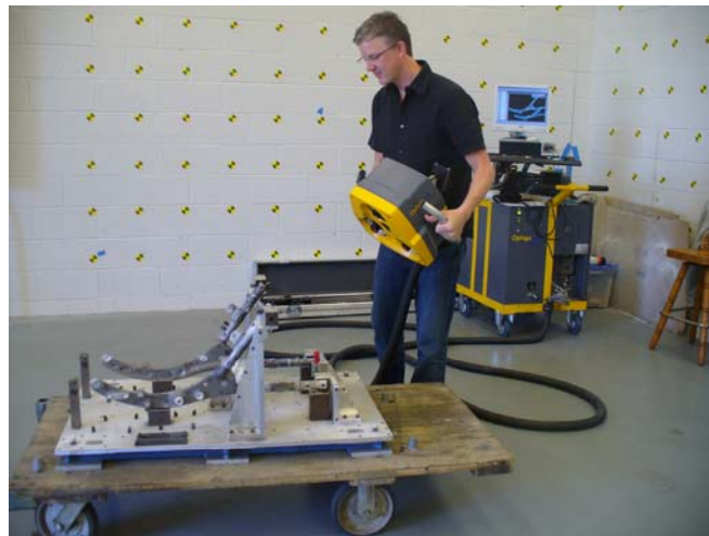
Figure 1. Sample Measurement of Part in Fixture Using 3D Coordinate Metrology
