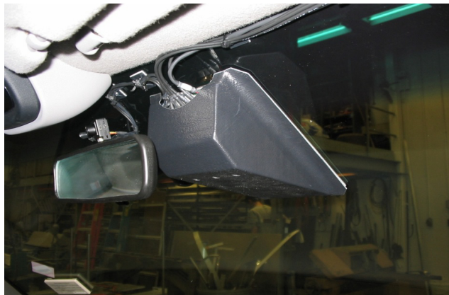
Figure 3: Three cameras, microphone, and IR illumination module
