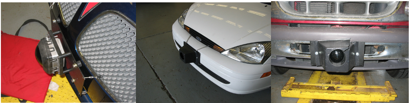
Figure 5: Forward radar: unshrouded (left), shrouded (middle), and cracked shroud with undamaged radar (right).
