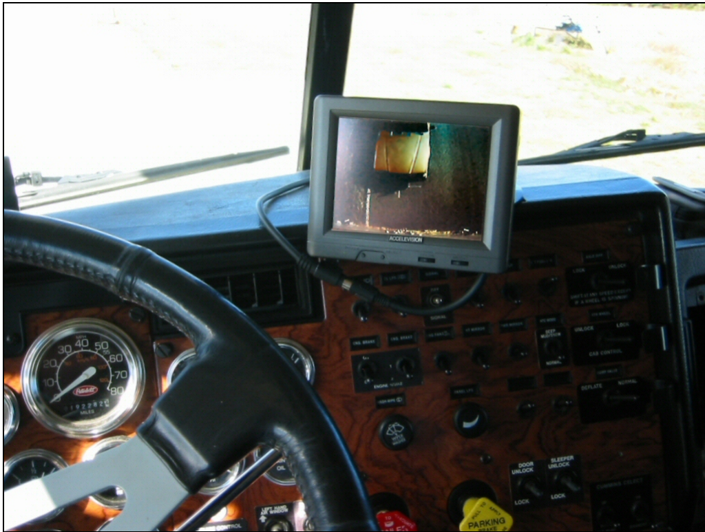
Figure 73. Dash monitor of Peterbilt during backing subtask with the trailer rear look-down C/VIS.
