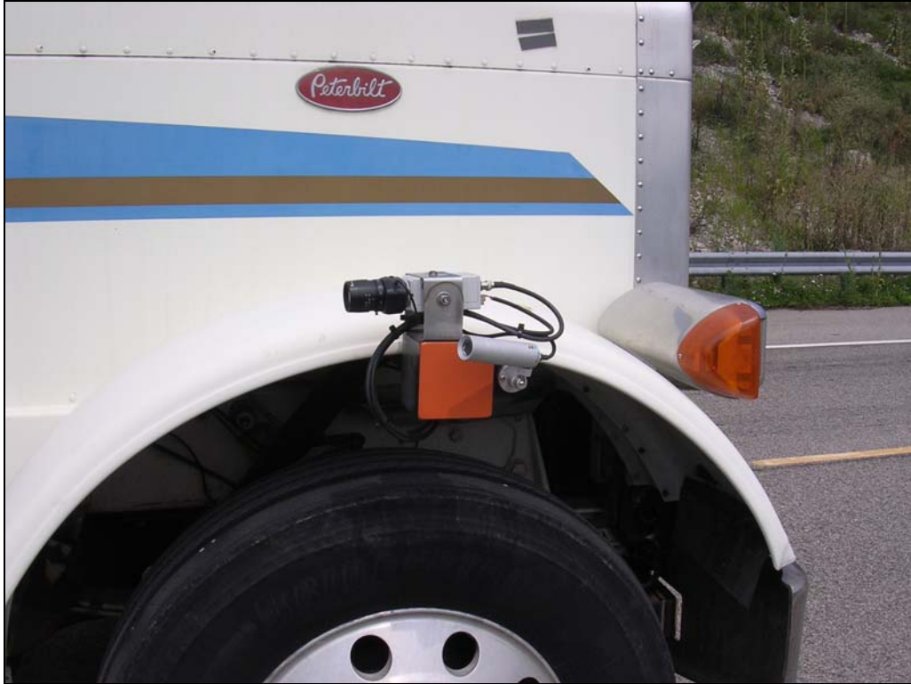
Figure 77. Passenger-side cameras at the front fender. The round camera is for the convex mirror surrogate, and the rectangular camera is for the west coast mirror surrogate.
