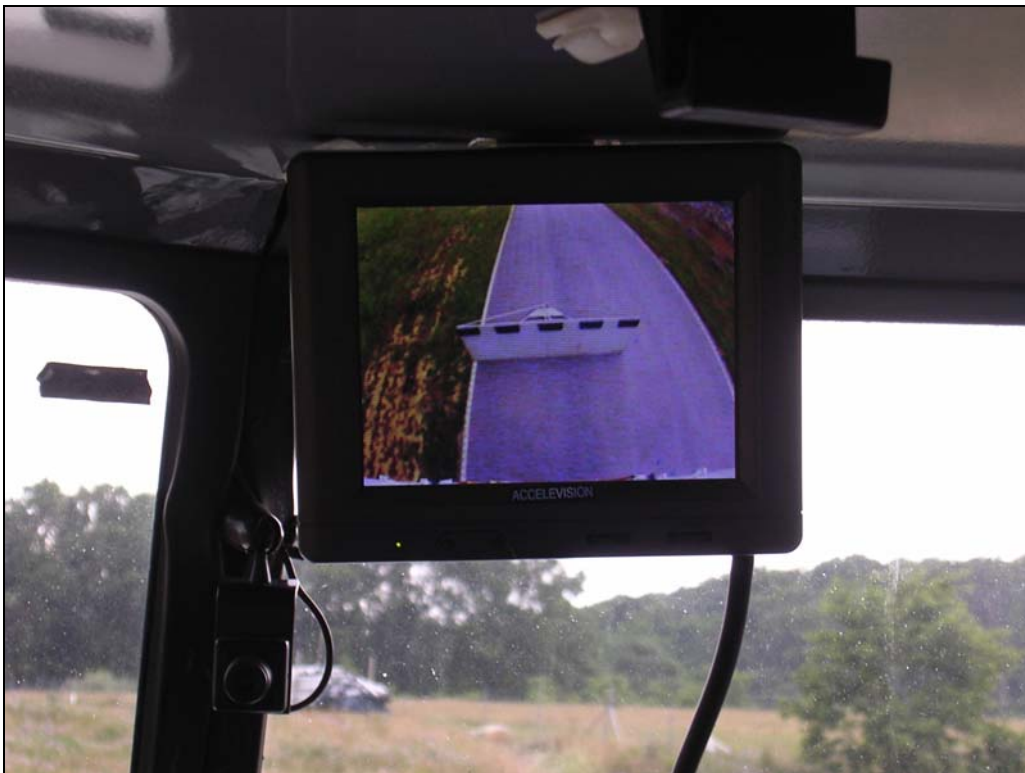
Figure 67. Monitor of Peterbilt during loading dock backing subtask for the wide-angle rear multipurpose trailer look-down C/VIS.
