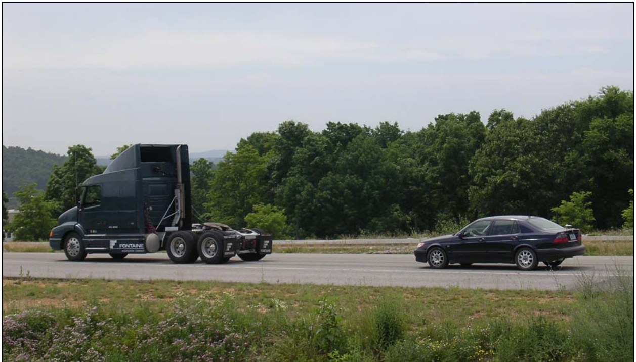
Figure 48. Volvo tractor and confederate automobile (Saab) used for the backing/bobtailing rear-view C/VIS experiment.
