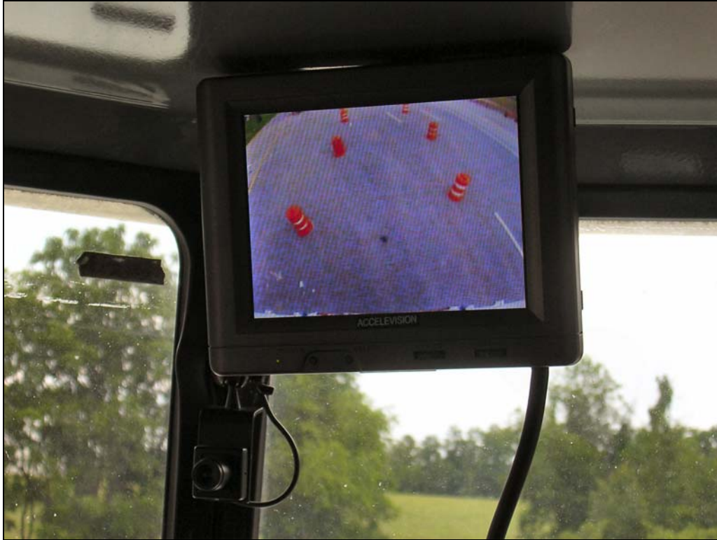
Figure 68. Monitor of Peterbilt during the S-curve backing subtask for the wide-angle rear multipurpose trailer look-down C/VIS.
