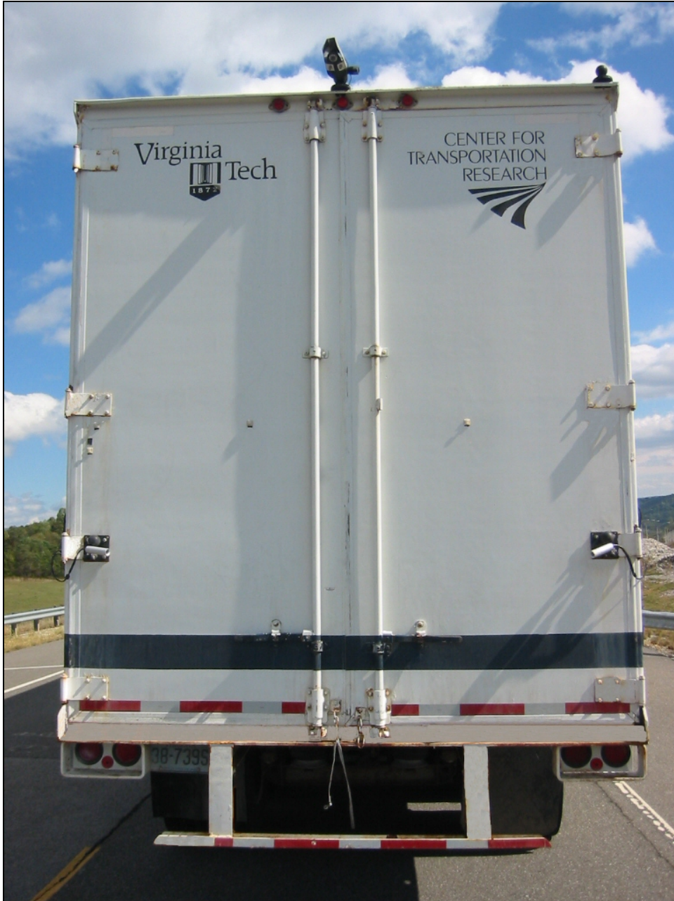
Figure 69. Back of trailer showing the three cameras used in Group 2 tests.
