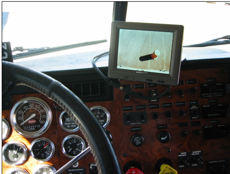
Figure 72. Dash monitor in the Peterbilt tractor used with the trailer rear look-down C/VIS.
