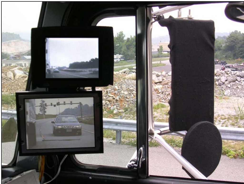
Figure 75. Passenger-side monitors mounted at the A-pillar. Note the covers over the mirrors, and note also that the upper monitor was hooded to reduce glare.
