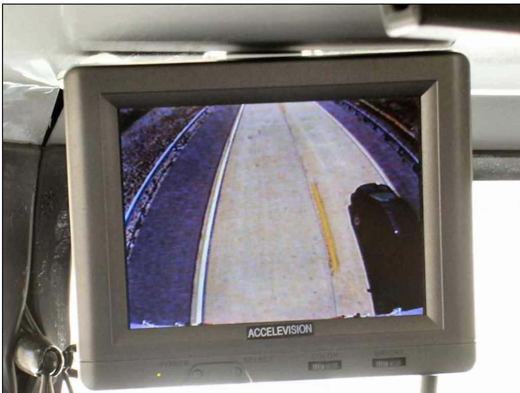
Figure 65. Monitor in Peterbilt with Saab in adjacent lane for the wide-angle rear multipurpose trailer look-down C/VIS.
