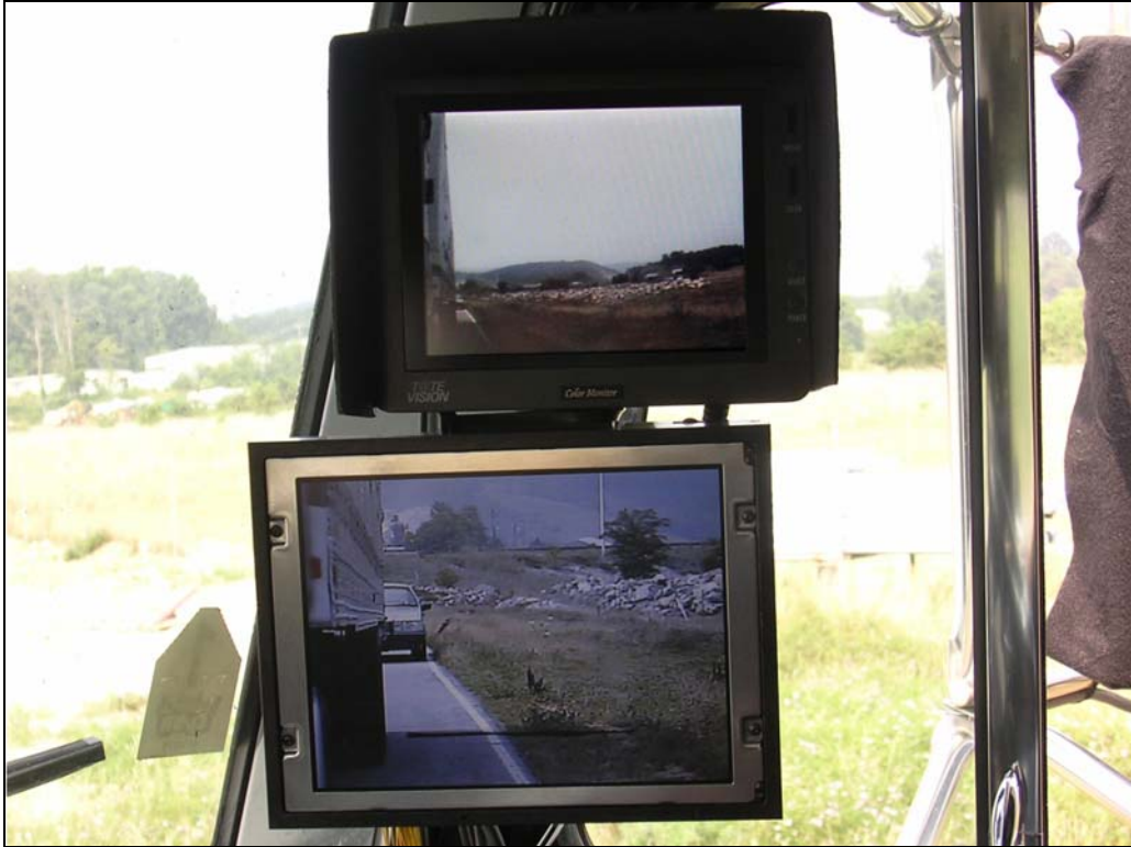
Figure 78. Typical view on the passenger-side monitors (for the convex and west coast mirror surrogates) during the task of backing to the parked car.
