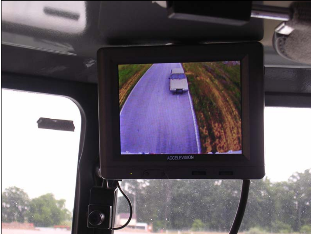
Figure 66. Monitor of Peterbilt during parking subtask for the wide-angle rear multipurpose trailer look-down C/VIS.
