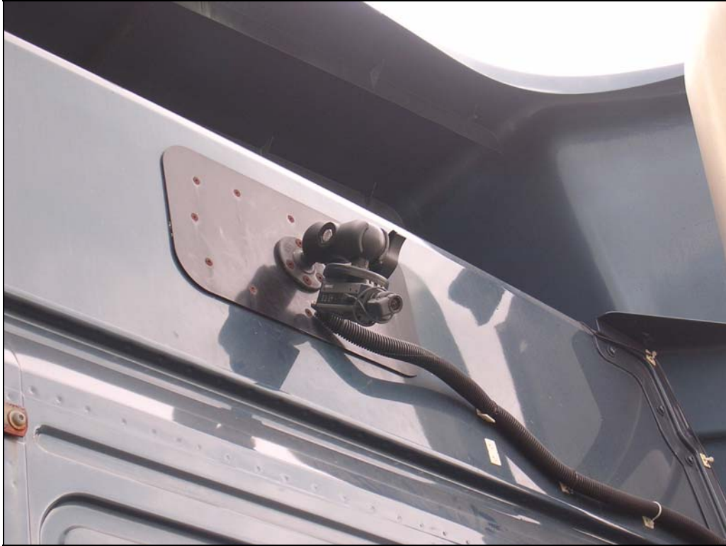
Figure 57. Rear of the Volvo tractor cab showing the rear-view C/VIS camera location.
