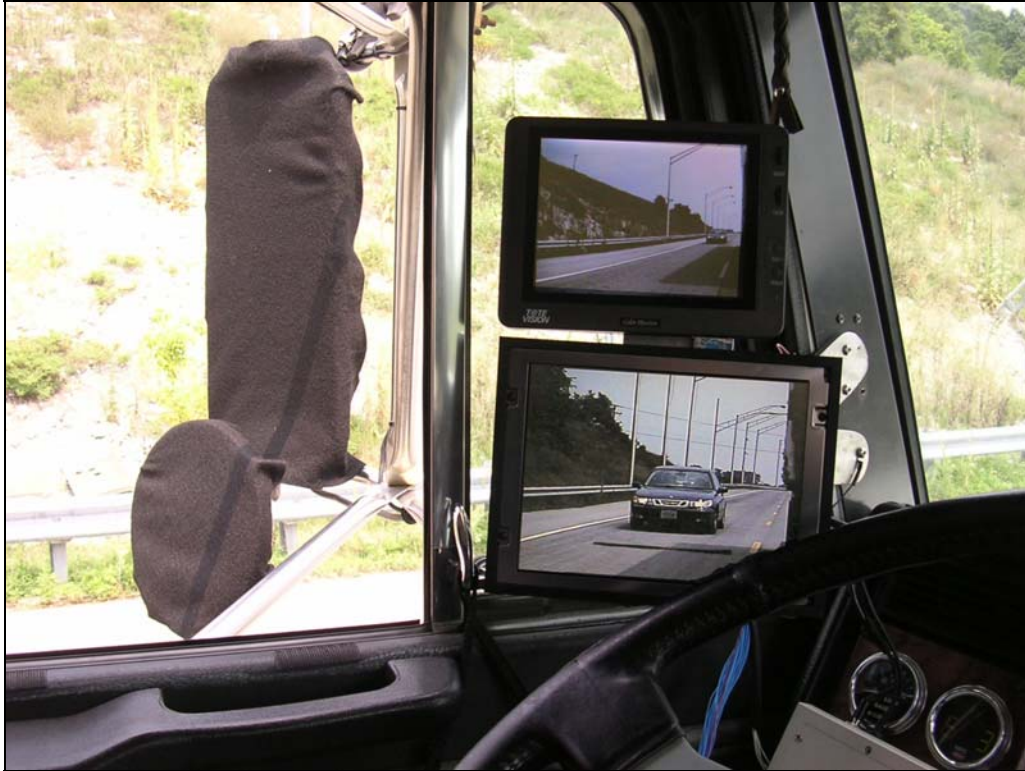
Figure 74. Driver-side monitors mounted at the A-pillar. Note the covers over the mirrors.
