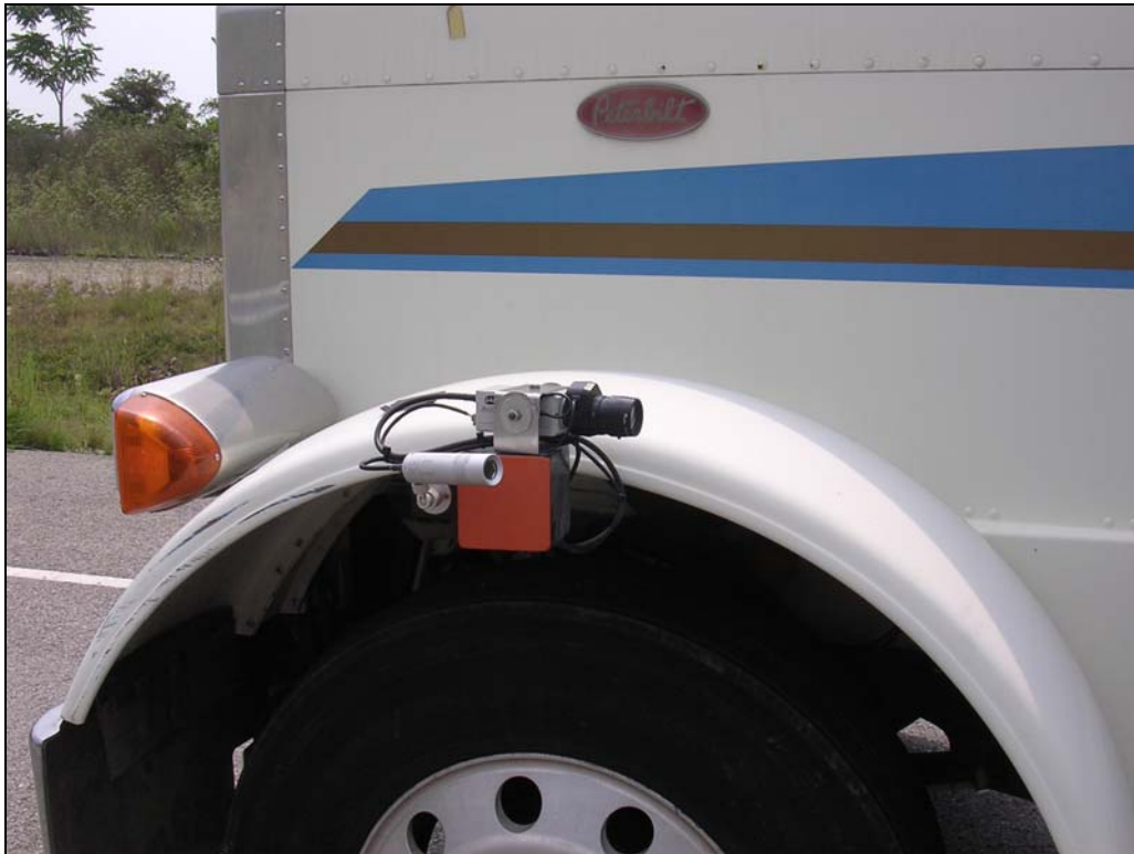
Figure 76. Driver-side cameras at the front fender. The round camera is for the convex mirror surrogate, and the rectangular camera is for the west coast mirror surrogate.
