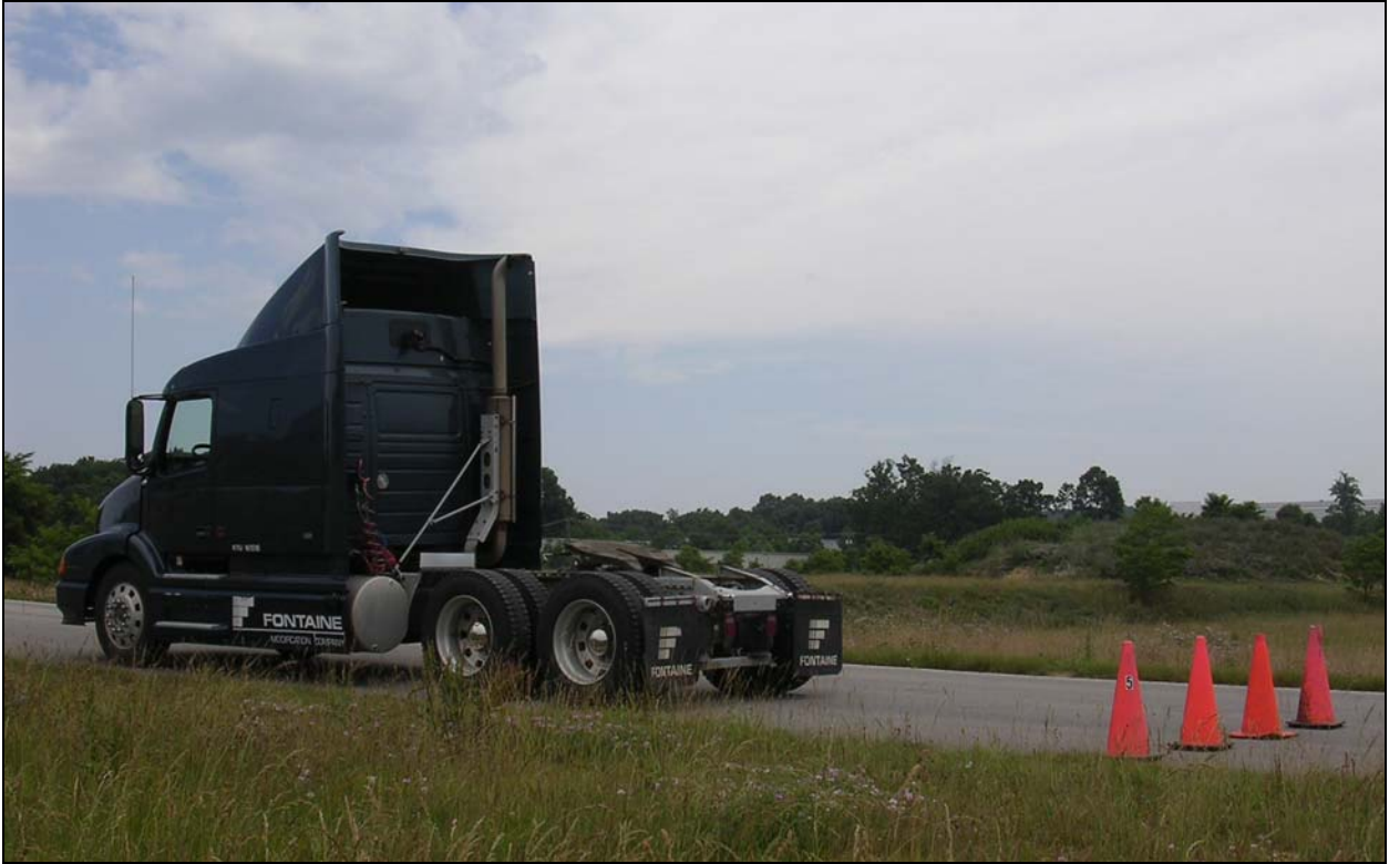
Figure 52. Volvo tractor backing to cone barrier.
