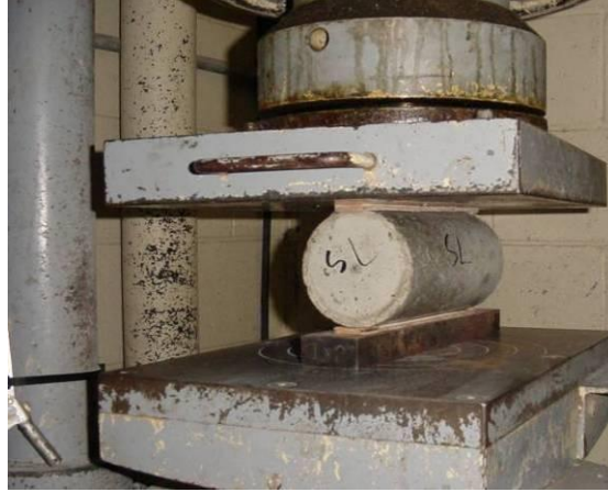
Figure 16. Splitting tensile strength test setup
