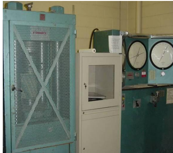
Figure 15. Forney 1 million pound compression machine
