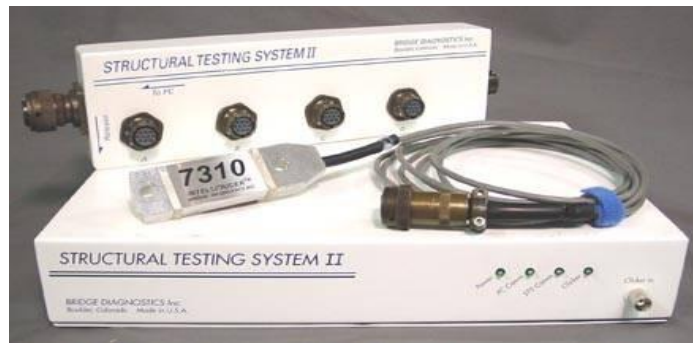
Figure 13. Structural testing system by Bridge Diagnostics Inc.
