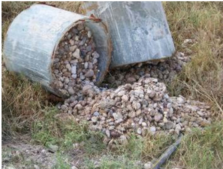
Figure 2.4.8 – 12" Sample obtained in the wet condition with No Cementation
