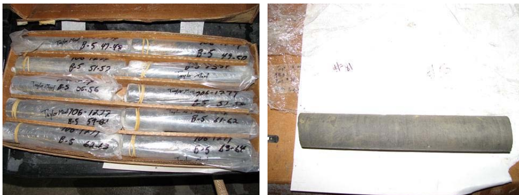
Figure 1.5.42 Taylor Marl cores prior to sample preparation
