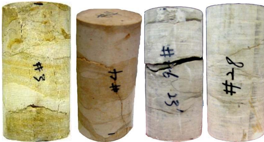
Figure 1.5.4 Failure modes of Edwards Limestone
