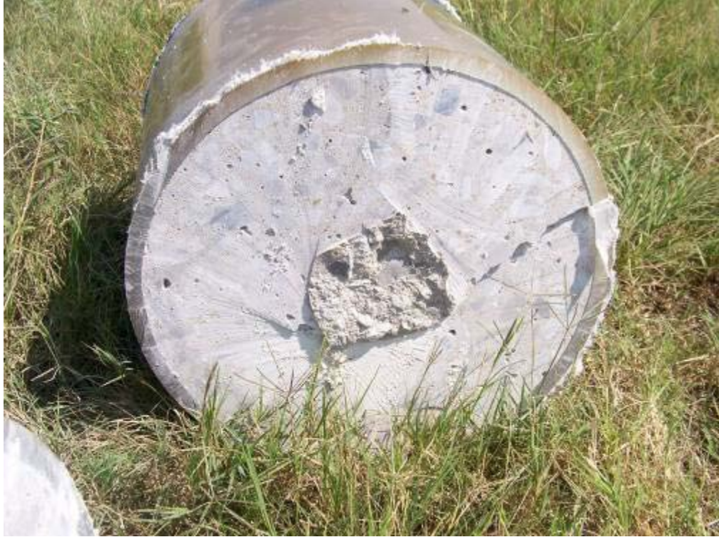
Figure 2.4.3 – 12” PVC pipe containing cured concrete
