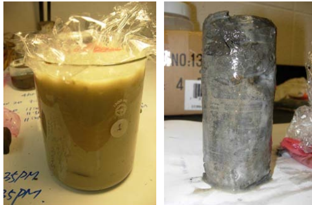
Figure 1.5.61 Shurry-soaked Navarro Shale specimen
