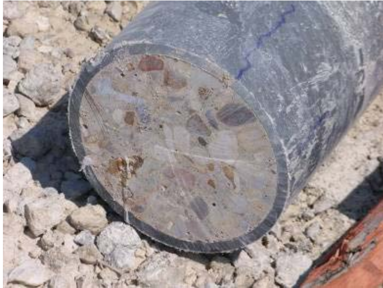
Figure 2.4.2 – 6" PVC pipe containing cured concrete
