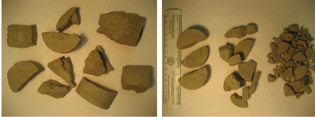
Figure 1.5.16 Austin Chalk chunks before and after two cycles of the slake durability test
