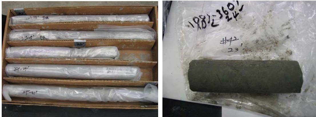
Figure 1.5.20 Del Rio Clay cores before sample preparation
