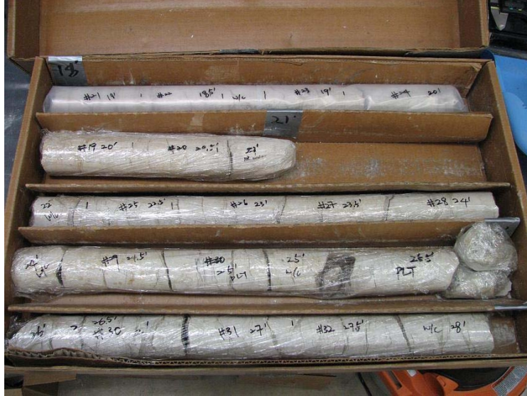
Figure 1.5.1 Edwards limestone cores before specimen preparation
