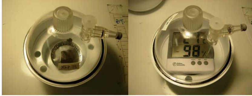
Figure 1.4.5 Eagle Ford Shale in a humidity controlled desiccators
