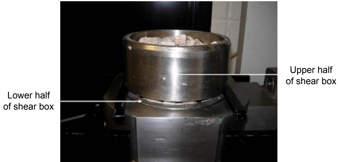
Figure 2.4.15 – Sample setup for the direct shear test
