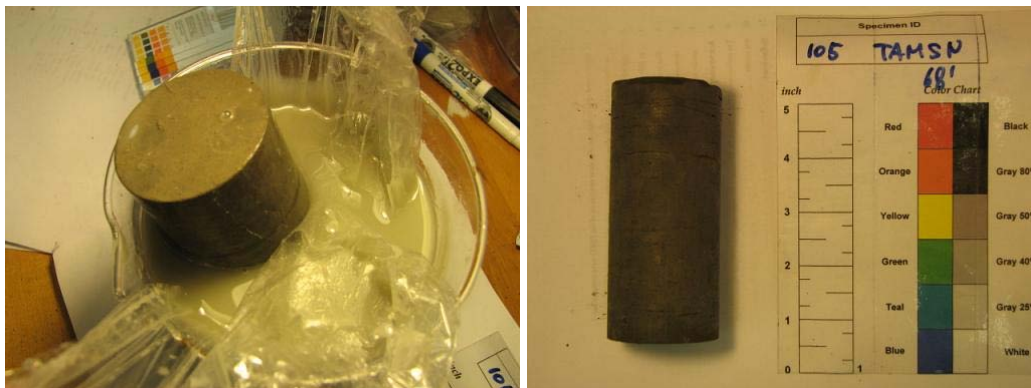
Figure 1.5.49 Taylor Marl slurry-soaked for 12 hours
