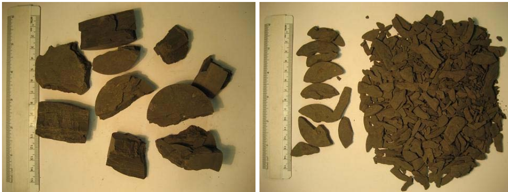
Figure 1.5.38 Eagle Ford Shale before and after the slake durability test (EFMSN)
