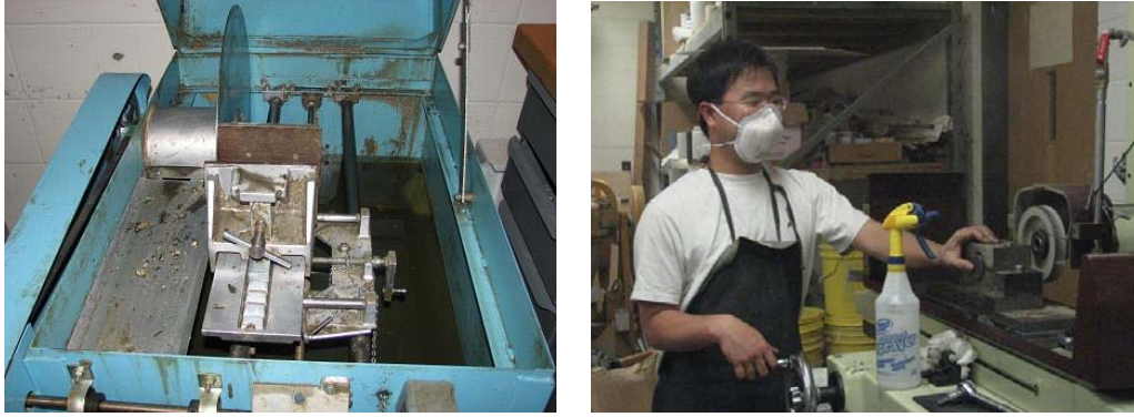
Figure 1.4.4 Slab saw (left) to initially cut the specimen to diameter to height ratio of 1:2, and the used grinder (right)
