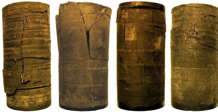
Figure 1.5.36 Failure modes of Eagle Ford Shale after multi-stage triaxial tests
