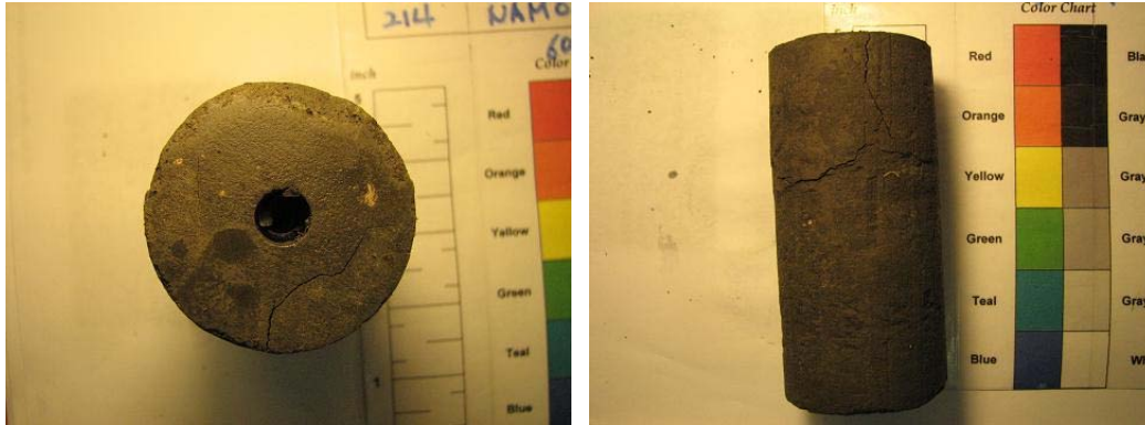
Figure 1.5.62 Navarro Shale specimen with hole after the triaxial test
