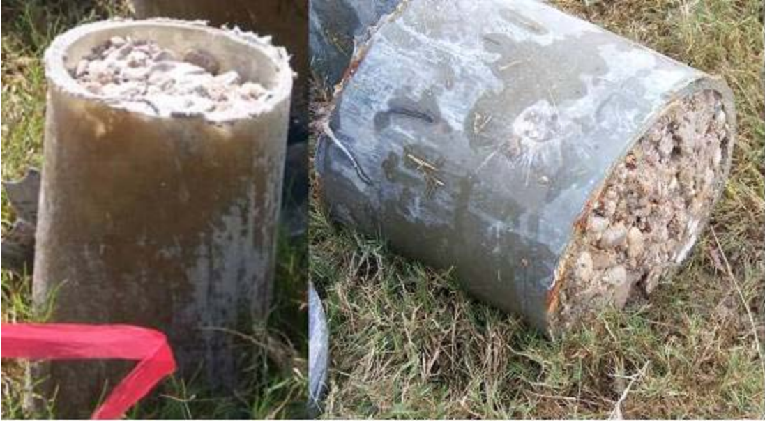
Figure 2.4.9 – Sample obtained in the wet condition with partial/weak cementation
