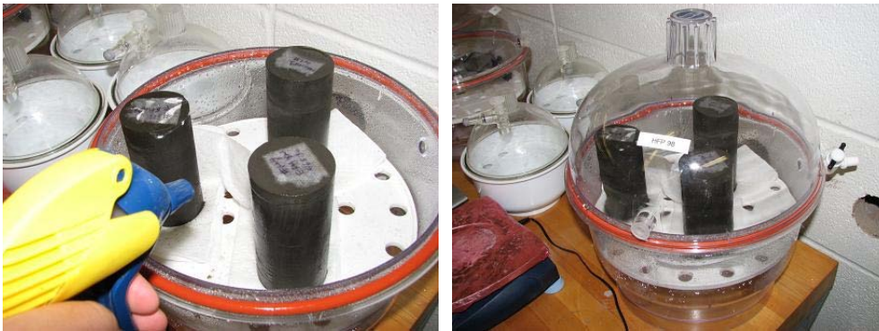
Figure 1.4.8 Water spraying to restore water content
