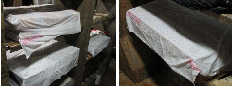
Figure 1.4.3 Moisture room to preserve cores at 100% relative humidity and 73°F
