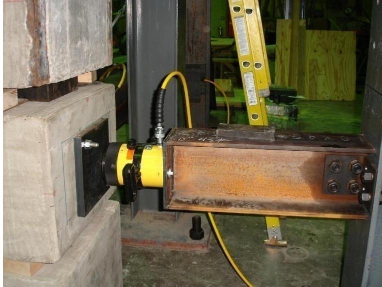
Figure 4.14 – Application of Transverse Load
