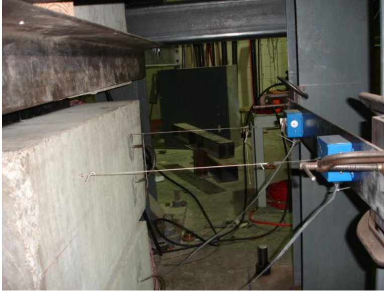
Figure 4.21 – Cable Extension Displacement Sensors – Longitudinal Direction
