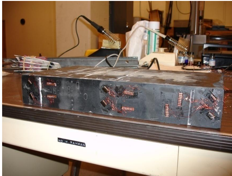
Figure 4.19 – Strain Gage Installed, 32-in. by 9-in. Bearing
