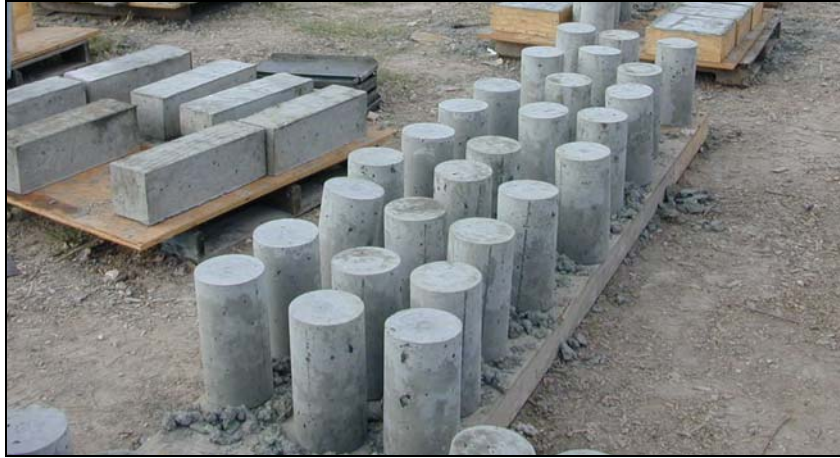
Figure 2.13 Demolded Field Cast Cylinders
