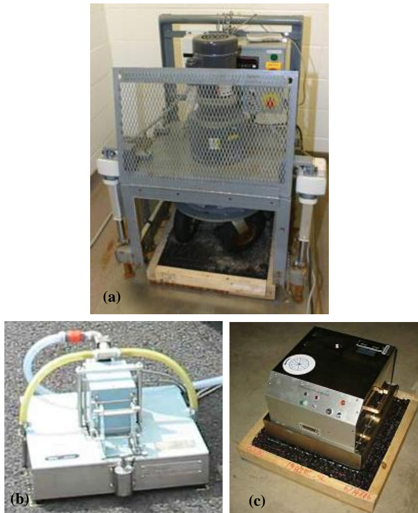
Figure 16. Polishing, friction and texture equipment: (a) CTPM, (b) DFT and (c) CTM
