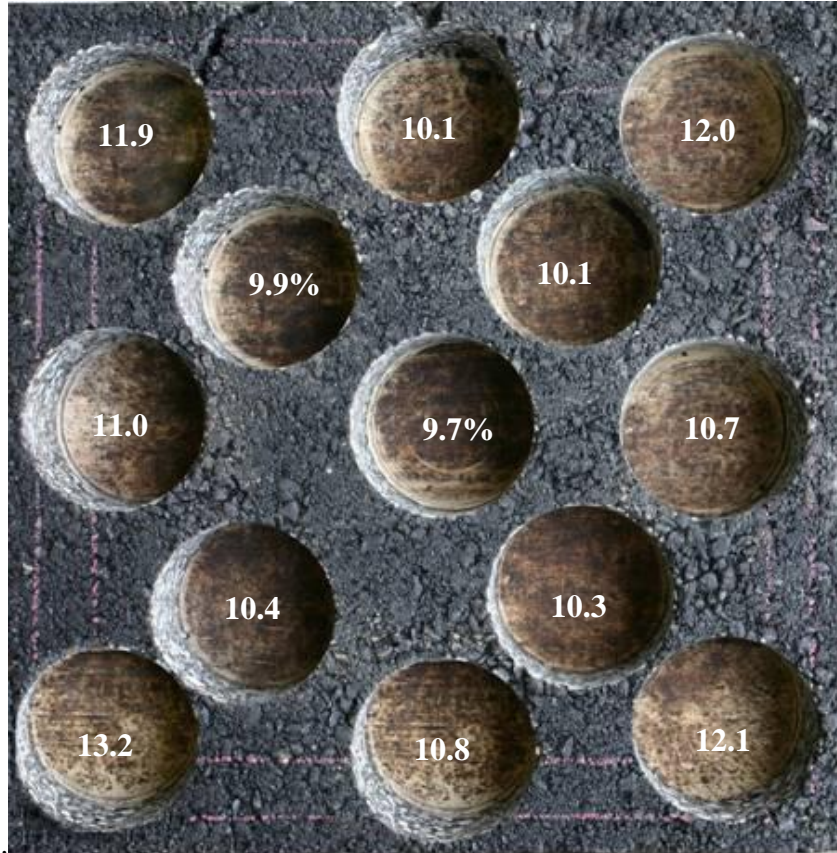
Figure 19. Air void content distribution
