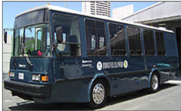
This fuel cell bus uses a 20 kW fuel cell from Hydrogenics. The bus originally was used in a yearlong demonstration at Hickman Air Force Base in Honolulu, Hawai'i. It has since entered into regular service on the base.
