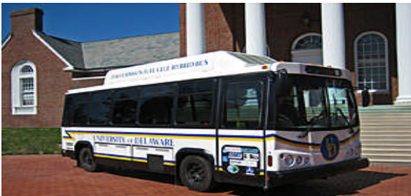
The University of Delaware's Department of Mechanical Engineering conducts research on two fuel cell buses that operate along normal campus routes. The 20 kW fuel cells are from Ballard Power Systems.
