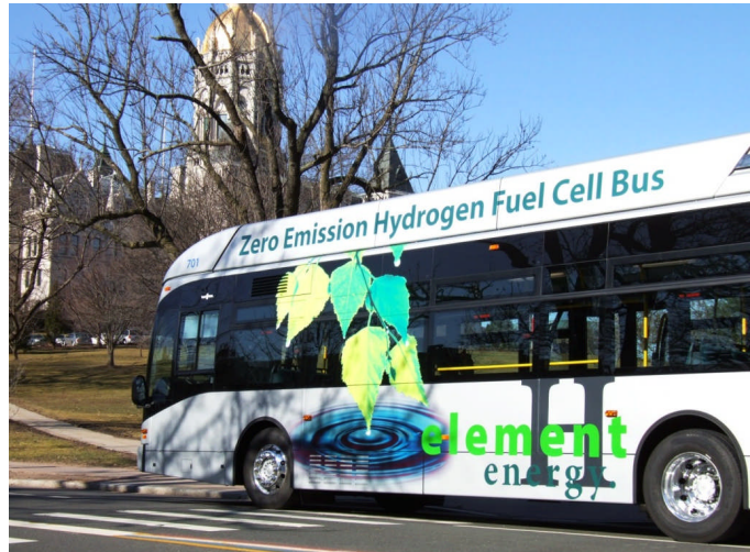
CTTransit operates a fuel cell bus in daily transit service. The vehicle is powered by a fuel cell from UTC Power, a Connecticut fuel cell manufacturer. The transit agency is planning deployment of additional fuel cell buses.
