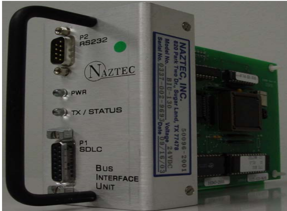
Figure 2. TS-2 Cabinet Enhanced BIU.
